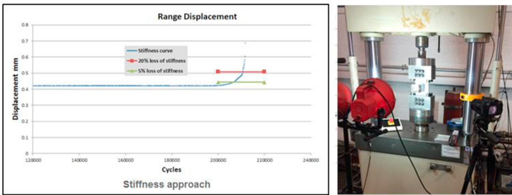
Fig.5. Crack initiation detection
