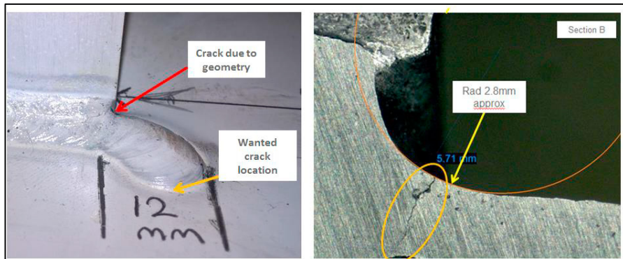
Fig.24. Weld defect crack
