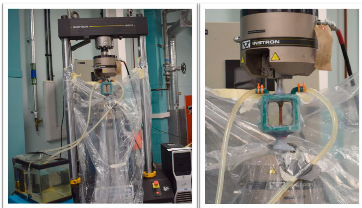
Fig.2 Corrosion system and detail of the chamber
