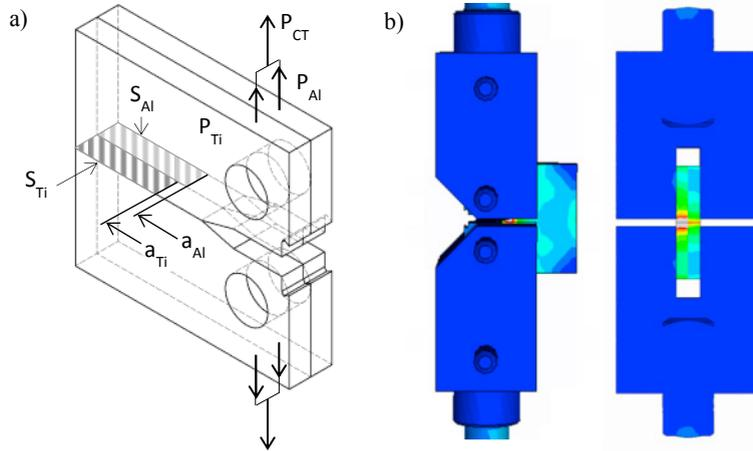
Fig. 7. Simplified model of specimen loading (a) and FEA analysis of loading system (b)
