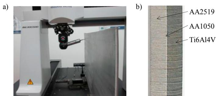
Fig. 2. AA2519-AA1050-Ti6Al4V layered material
