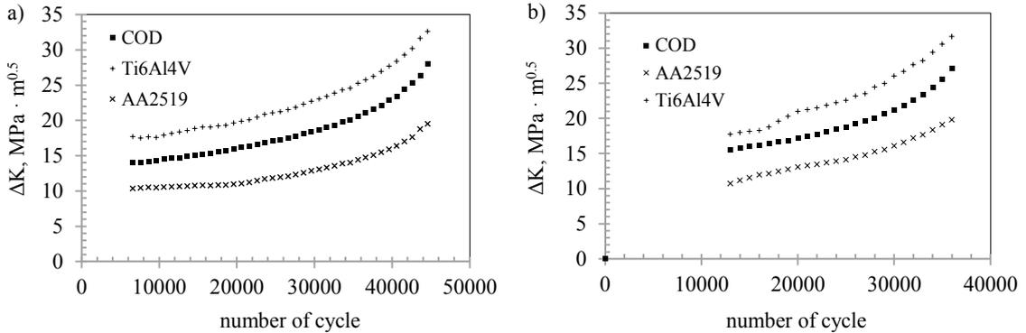
Fig. 8. Changes in  $\Delta K$  value for both layers (Ti6Al4V, AA2519) and whole specimen (COD) for: a) crack initiation in Ti6Al4V layer, b) crack initiation in AA2519 layer.
