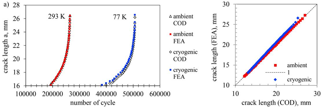
Fig. 9. Crack length for ambient (293 K) and cryogenic (77 K) conditions (a). Comparison of crack length determined for the same number of cycle by the compliance method (COD) and the hybrid method (FEA) (b).
