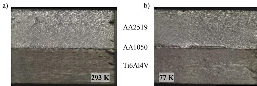
Fig. 10. Images of fracture surface: a) for ambient conditions, b) for cryogenic conditions.
