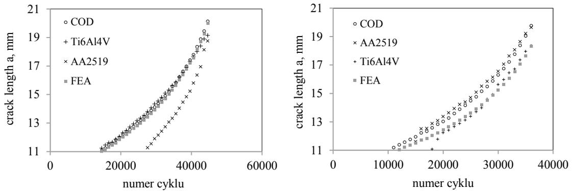
Fig. 6. Examples of measured and calculated crack length in CT specimens for: a) crack initiation in Ti6Al4V layer, b) crack initiation in AA2519 layer. ‘Ti6Al4V’ - crack length measured on the titanium alloy surface, ‘AA2519’ - crack length measured on the aluminum alloy surface, ‘COD’ - crack length determined by the compliance method, ‘FEA’ - crack length determined by the hybrid, experimental-numerical method
