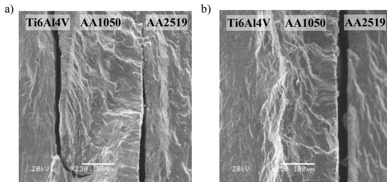
Fig. 11. Examples of layers delaminations under cryogenic conditions: a) delamination between the AA1050 and Ti6Al4V, b) AA1050 and AA2519
