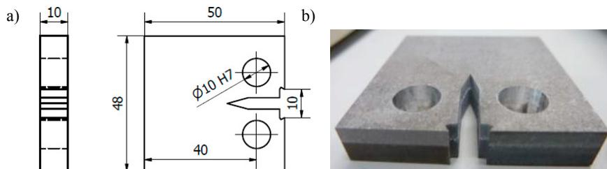
Fig. 3. AA2519-AA1050-Ti6Al4V layered material: a) dimensions, b) layers configuration in the CT specimen.
