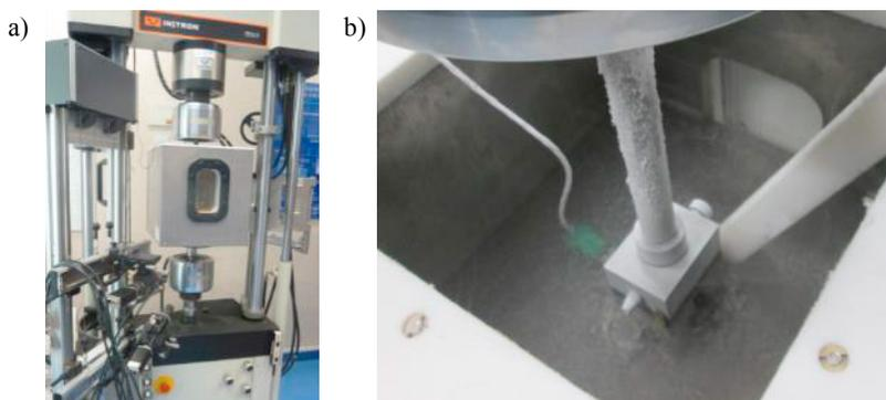
Fig. 4. Research stand: a) general view, b) specimen immersed in the liquid nitrogen
