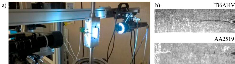
Fig. 5. Crack length measurement system: a) general view of FatigueVIEW system, b) specimen surface images.
