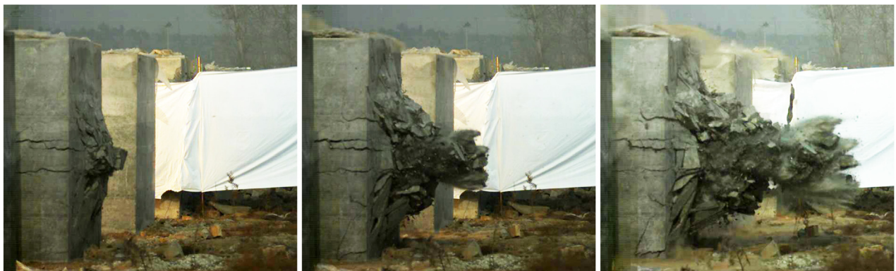
(b) The perforation progress of shear plugging
