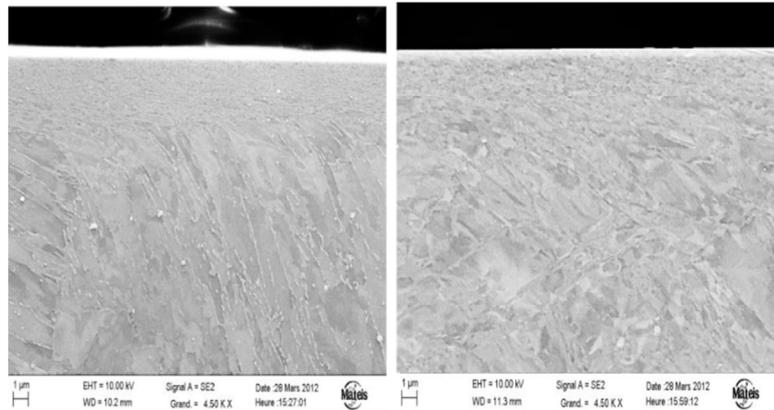
Figure 4: Surface layer generated by turning (left) and ball burnishing (right) [5]
