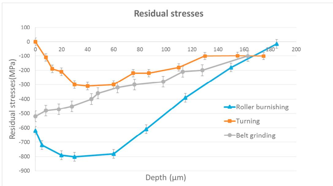
Figure 3: Residual stress gradients for the 3 sets of samples
