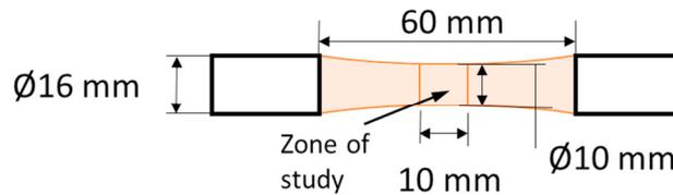
Figure 2: Bending test fatigue samples
