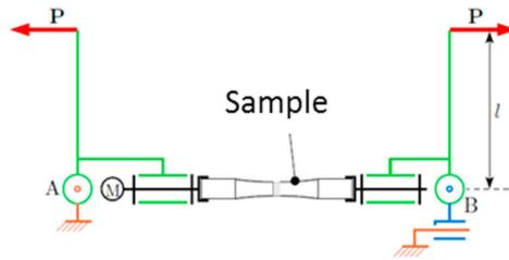
Figure 6: Rotary bending fatigue system
