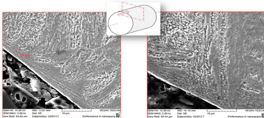
Figure 5: SEM observation of the surface layer after turning (left) and belt grinding (right)
