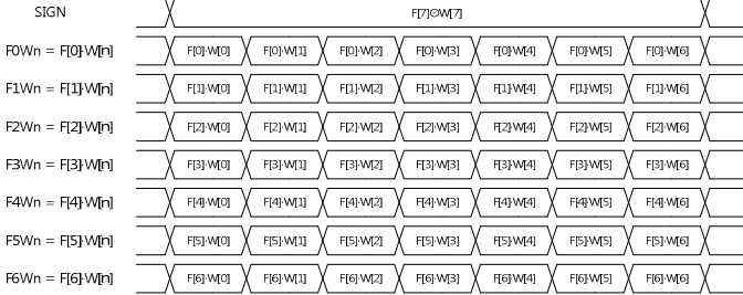
Fig. 2. Output sequence of Bit Multiplier
