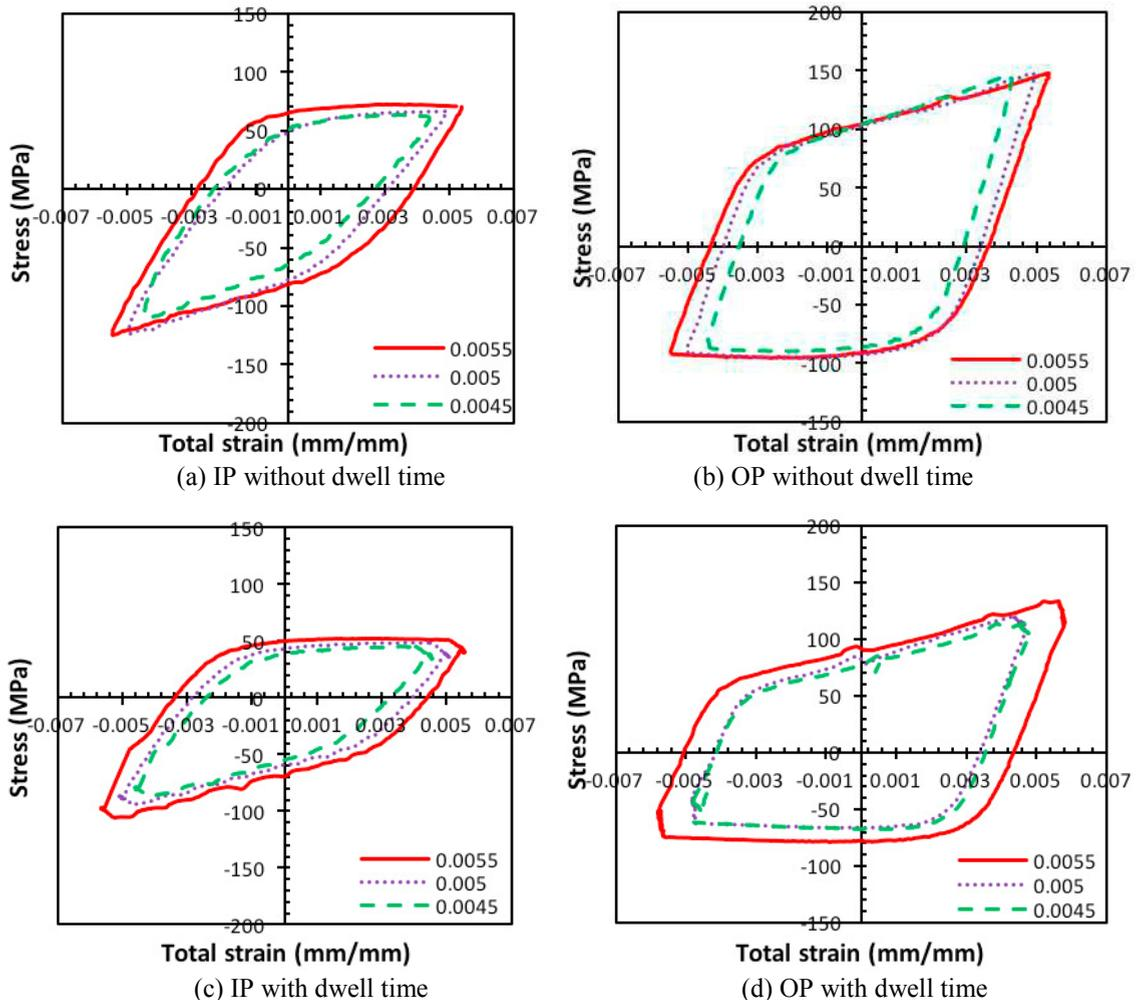
Fig. 13. Hysteresis loops at the stabilized cycles for (a) IP loading, (b) OP loading, (c) IP loading with dwell time, and (d) OP loading with dwell time, tested at 3 different strain amplitudes.
