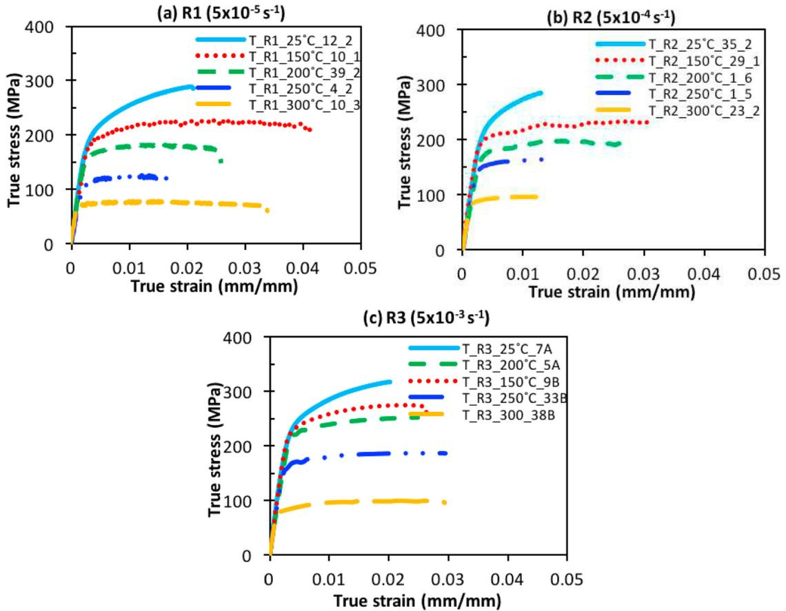
Fig. 5. Monotonic stress-strain curves at various temperatures with strain rate of (a)  $5 \times 10^{-5} \text{ s}^{-1}$ , (b)  $5 \times 10^{-4} \text{ s}^{-1}$  and (c)  $5 \times 10^{-3} \text{ s}^{-1}$ .
