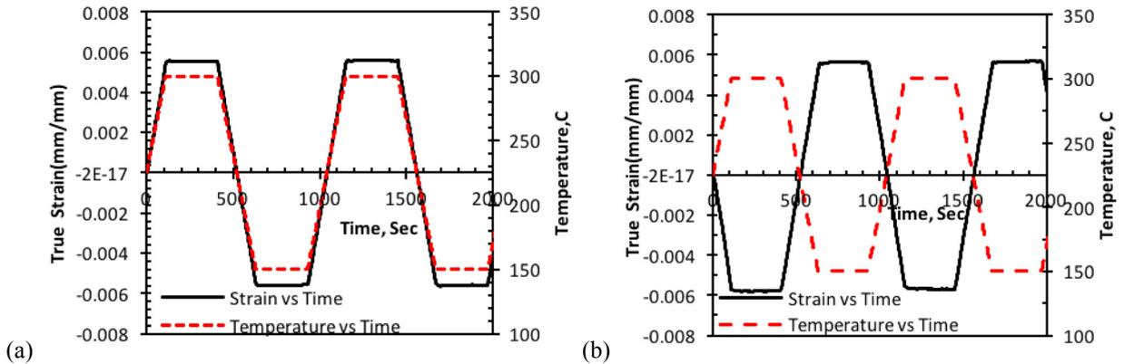
Fig. 4. Loading profiles of (a) in-phase and (b) out-of-phase TMF with 300s dwell time.
