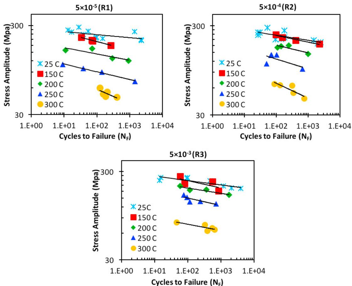
Fig. 11. Stress amplitude vs. fatigue life at various temperatures with strain rates of (a)  $5 \times 10^{-5} \text{ s}^{-1}$ , (b)  $5 \times 10^{-4} \text{ s}^{-1}$  and (c)  $5 \times 10^{-3} \text{ s}^{-1}$ .
