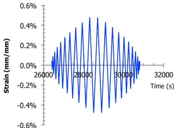
Fig. 3. Incremental strain block used for cyclic tests.
