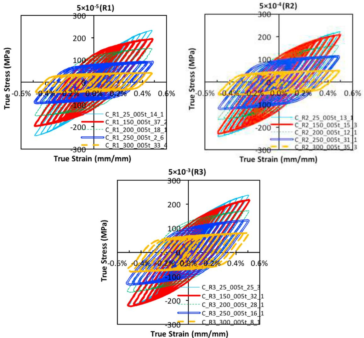
Fig. 8. Stabilized cyclic behaviors at various temperatures with strain rates of (a)  $5 \times 10^{-5} \text{ s}^{-1}$ , (b)  $5 \times 10^{-4} \text{ s}^{-1}$  and (c)  $5 \times 10^{-3} \text{ s}^{-1}$ .
