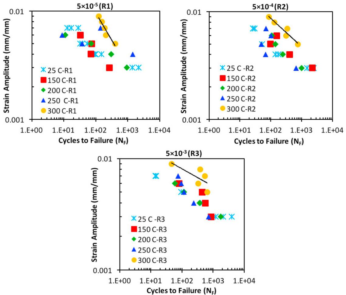
Fig.10. Strain amplitude vs. fatigue life at various temperatures with strain rates of (a)  $5 \times 10^{-5} \text{ s}^{-1}$ , (b)  $5 \times 10^{-4} \text{ s}^{-1}$  and (c)  $5 \times 10^{-3} \text{ s}^{-1}$ .
