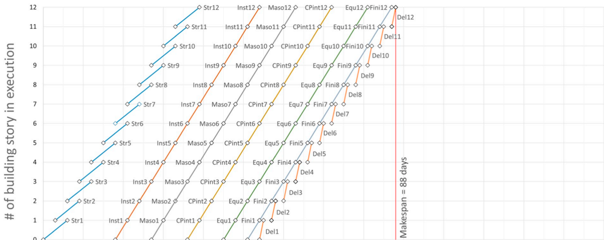
Fig. 9. Model 8 with multiple crews, non-accelerated routine, and non-continuity condition.
