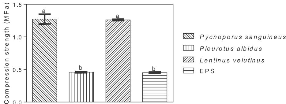
**Fig. 6.** Compression strength for biofoams of *Pycnoporus sanguineus*, *Pleurotus albidus*, *Lentinus velutinus* as compared with EPS <sup>a, b, c</sup>. Values were determined in triplicate. Same letters mean there are no significant differences at 5% ( $p < 0.05$  for the Tukey test).
