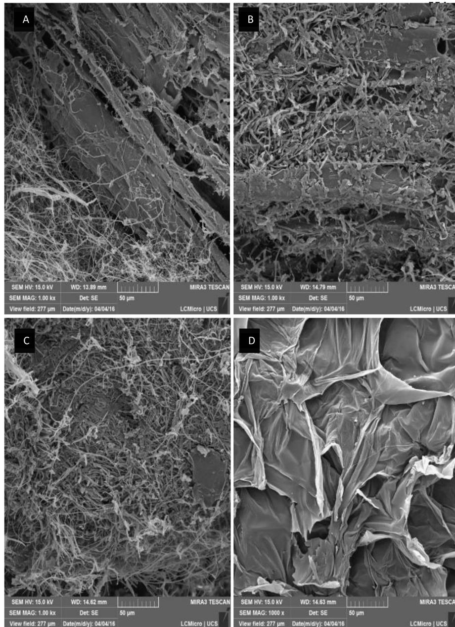
**Fig. 3.** FE SEM Micrographs of (A) *Pycnoporus sanguineus*, (B) *Pleutorus albidus*, (C) *Lentinus velutinus* biofoams and (D) of EPS.
