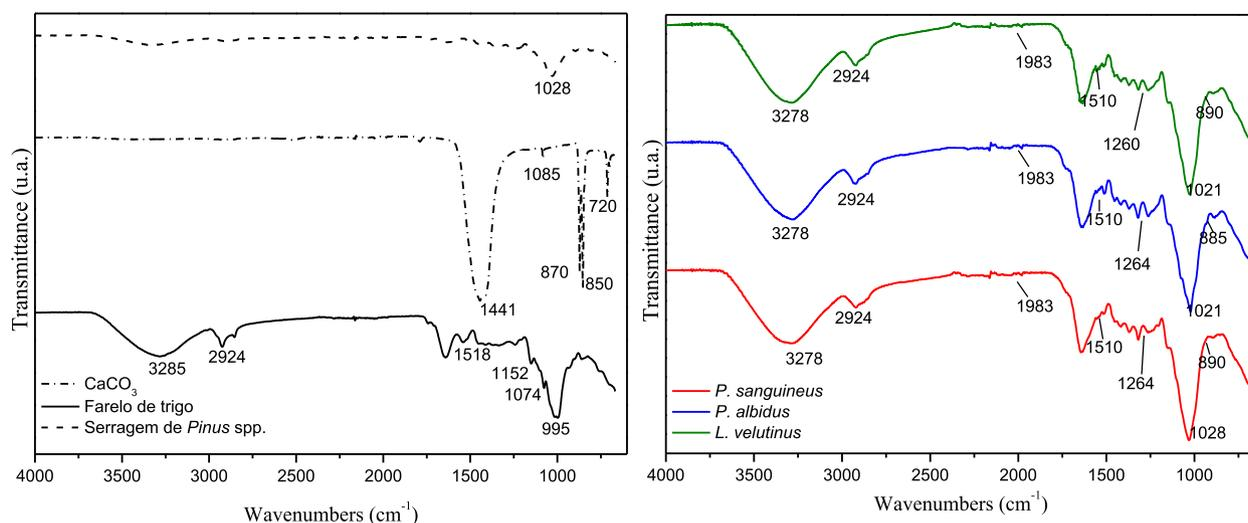
Fig. 5. Infrared spectra (A) of  $\text{CaCO}_3$ , wheat bran and sawdust substrates and (B) biofoams samples from *Pycnoporus sanguineus*, *Pleurotus albidus*, *Lentinus velutinus*.
