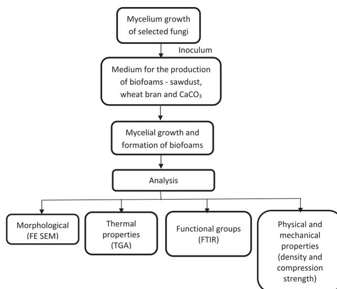
Fig. 1. Flow chart of the activities carried out for the production and analysis of biofoams.
