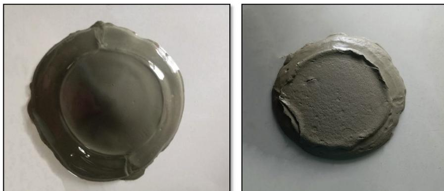
Fig. 3. Comparison of spread diameters from the mini slump test: (a) C1-0.4 suspension with a 14.15 cm flow diameter; (b) AAF-3.0 suspension with a 14.62 cm flow diameter.
