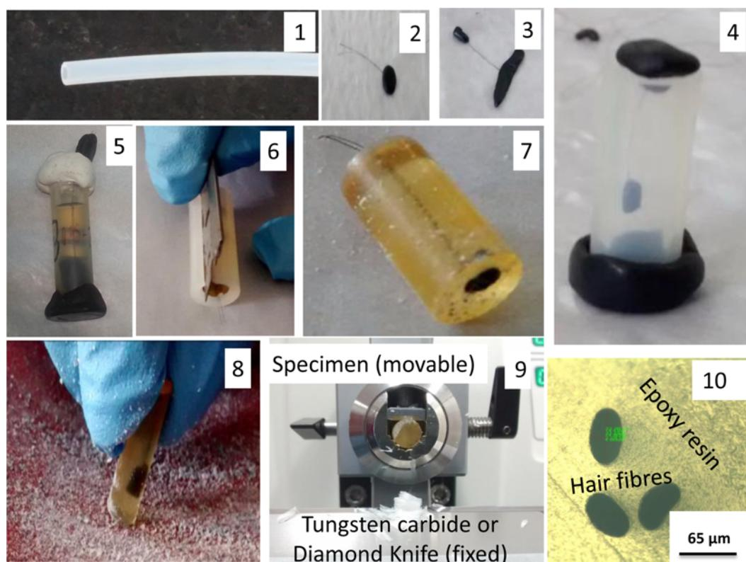
**Figure 1.** Images (1-9) correspond to sample preparation for nanoindentation test. Hair samples are embedded in agar epoxy resin using silicone mold (1) and clay (2-4). After curing of liquid epoxy resin (5), epoxy block was released from the mold using a razor blade (6) followed by smooth polishing (8, 9) using a rotary microtome (thin slices). Image (10) shows such a smooth epoxy block in which three fiber cross-sections are visible.
