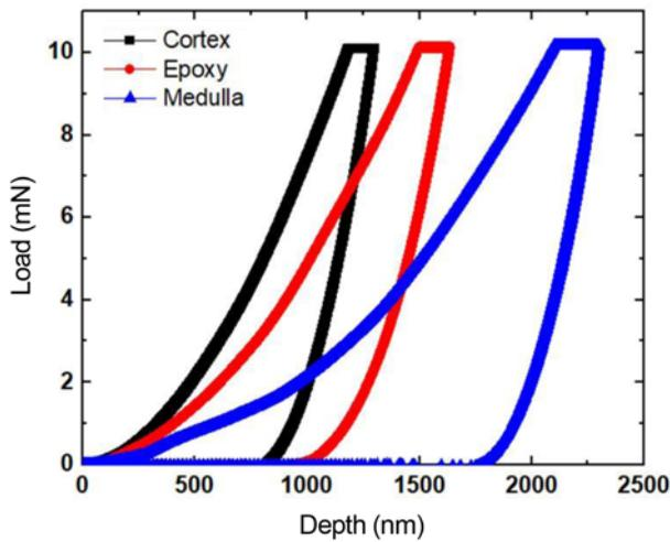
**Figure 3.** Typical load-depth graphs of nanoindentation test performed on hair fiber cortex and medulla regions. Since hair samples were embedded in epoxy resin, indents were also placed on surrounding epoxy.
