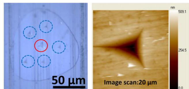
**Figure 2.** Left image shows five residual indentation impressions (dotted circle) on cortex region and one residual indentation imprint (solid circle) on medulla. Implanted knife markers due to sectioning are also visible on hair cross section. Right image shows one residual indentation imprint of Berkovich diamond indenter on cortex region which was taken using a scanning probe microscope.
