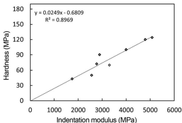
**Figure 5.** Correlation between hardness and indentation modulus found for medulla data indicating the variation in nanocomposite structure of macrofibrils especially orientation of helical intermediate filaments (microfibrils) in medulla.
