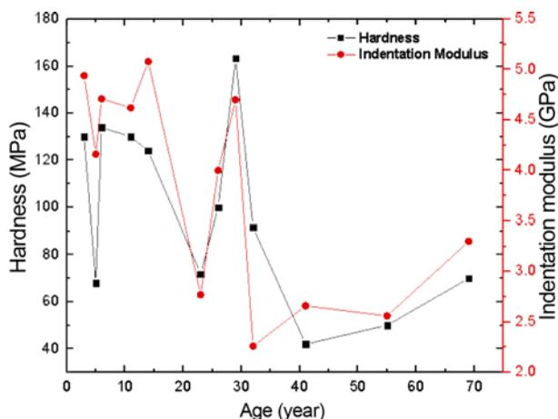
**Figure 8.** Variation of hardness and indentation modulus of hair samples (medulla) with respect to age.
