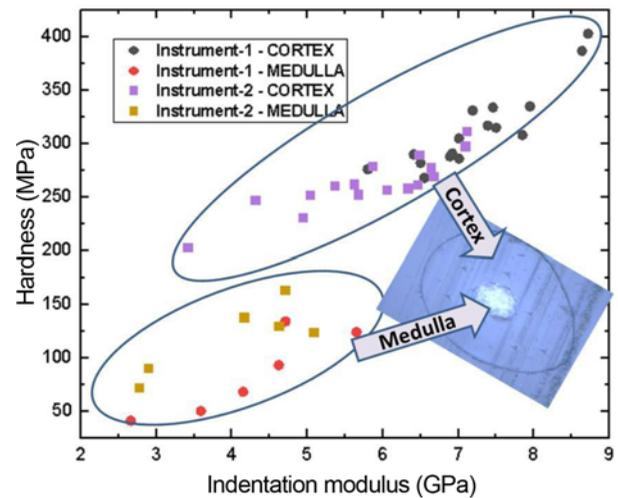
**Figure 4.** Variation of hardness and indentation modulus of hair samples with respect to cortex and medulla. Here nanoindentation on hair cross sections was performed using two instruments (Instrument-1 & Instrument-2) to validate the results.
