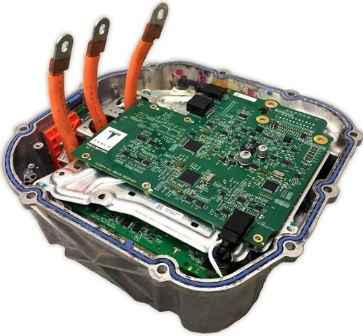
Fig. 5: Tesla Model S dual motor rear drive unit inverter.
