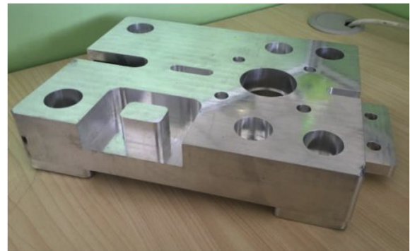
Fig. 11. Test part that has been machined.
