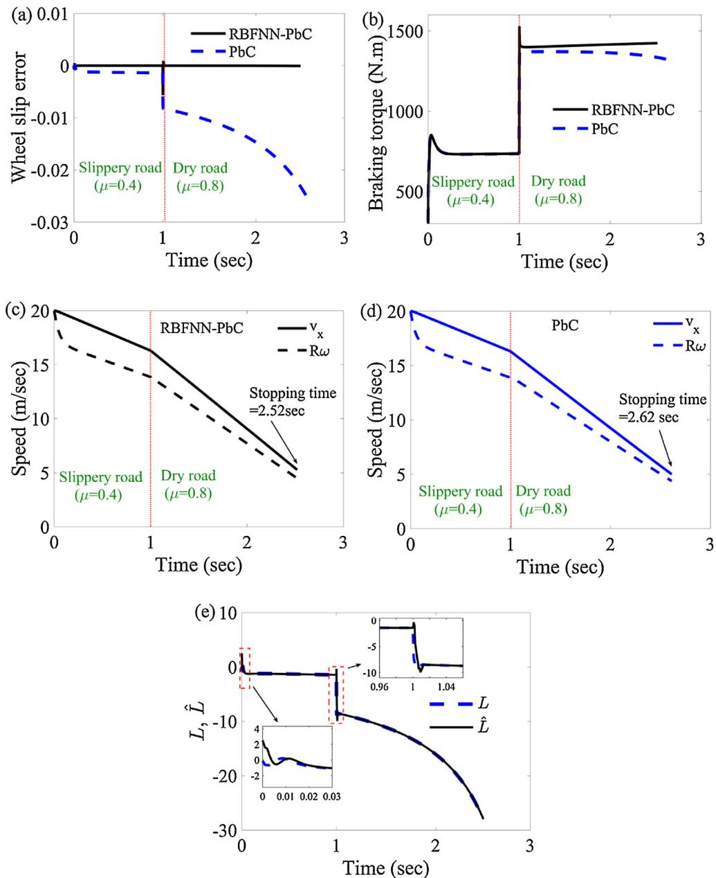
**Fig. 9.** Comparison of performances of the PbC and RBFNN-PbC for maneuver 3: (a) wheel slip tracking error, (b) braking torque, (c) and (d) wheel and vehicle speed and (e)  $L$  and  $\hat{L}$ .
