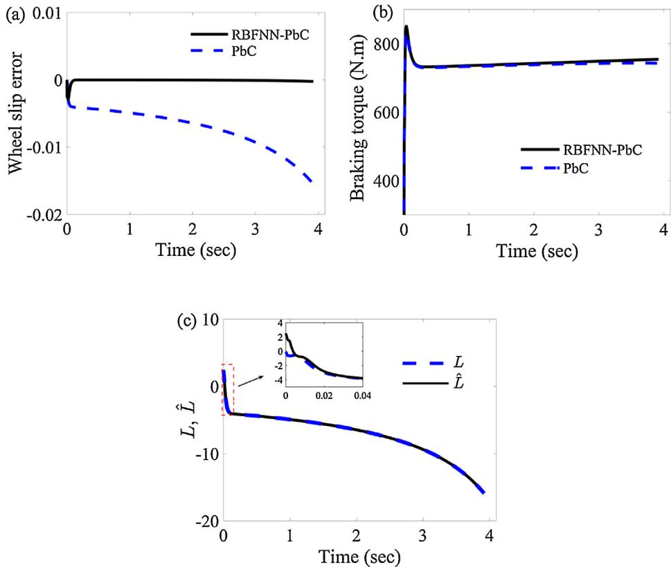
**Fig. 8.** Comparison of performances of the PbC and RBFNN-PbC for maneuver 2: (a) wheel slip tracking error (b), braking torque and (c)  $L$  and  $\hat{L}$ .
