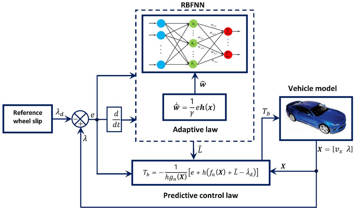
**Fig. 3.** Overall structure of the proposed control system.
