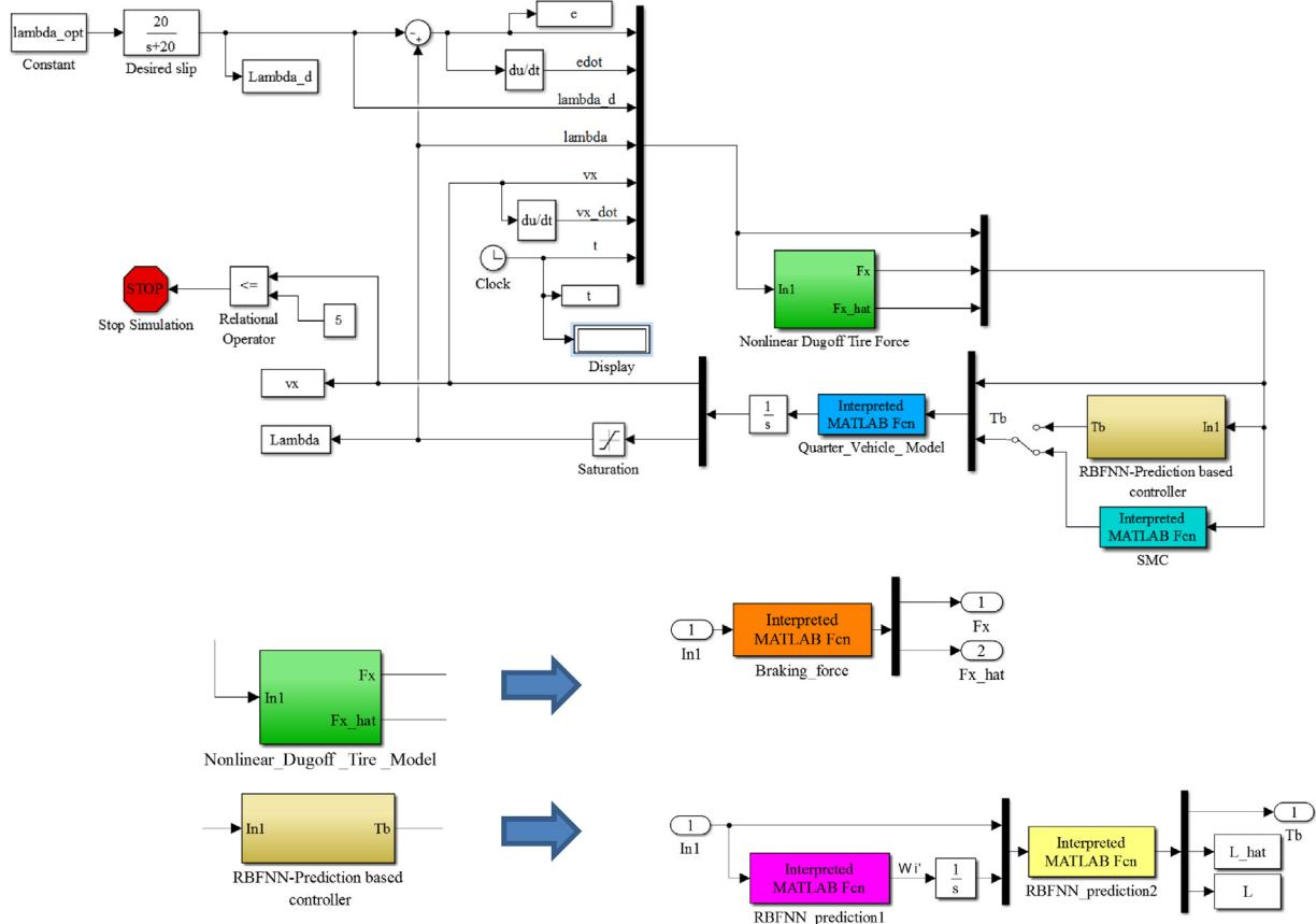
**Fig. 4.** The Simulink scheme of the proposed control system.
