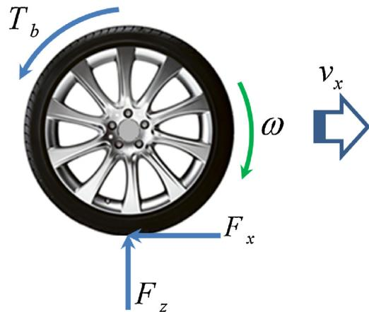
**Fig. 1.** Wheel free body diagram.
