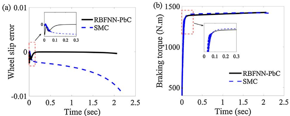
**Fig. 10.** Comparison of performances of the RBFNN-PbC and SMC for maneuver 1: (a) wheel slip tracking error and (b) braking torque.
