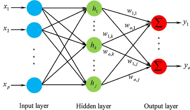
**Fig. 2.** Schematics of the RBFNN with multiple outputs.
