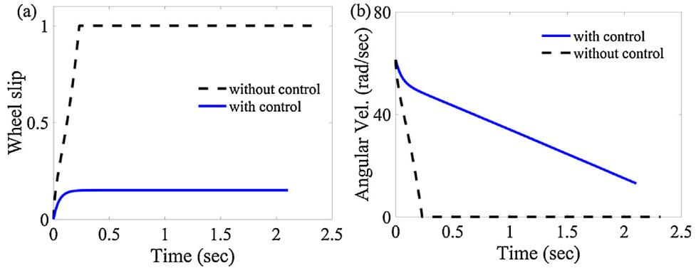
**Fig. 5.** Comparison of the responses of the controlled and uncontrolled vehicle during braking (a) wheel slip (b) wheel angular velocity.
