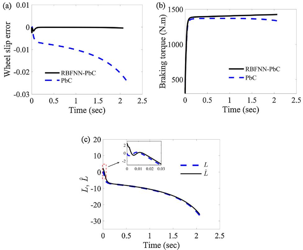
**Fig. 6.** Comparison of performances of the PbC and RBFNN-PbC for maneuver 1: (a) wheel slip tracking error, (b) braking torque and c)  $L$  and  $\hat{L}$ , maneuver 1.
