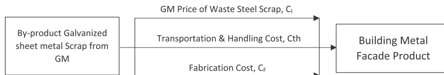
Fig. 5. Capital cost flowchart for making a building metal facade product by reusing steel scrap material.
