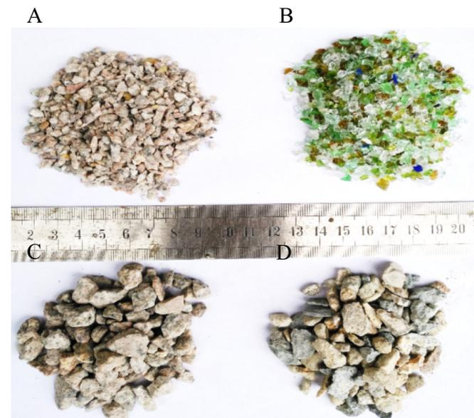
**Fig. 1.** Appearance of aggregates A: NA (2.36–5 mm), B: WGC (2.36–5 mm), C: NA (5–10 mm), D: RCA (5–10 mm).
