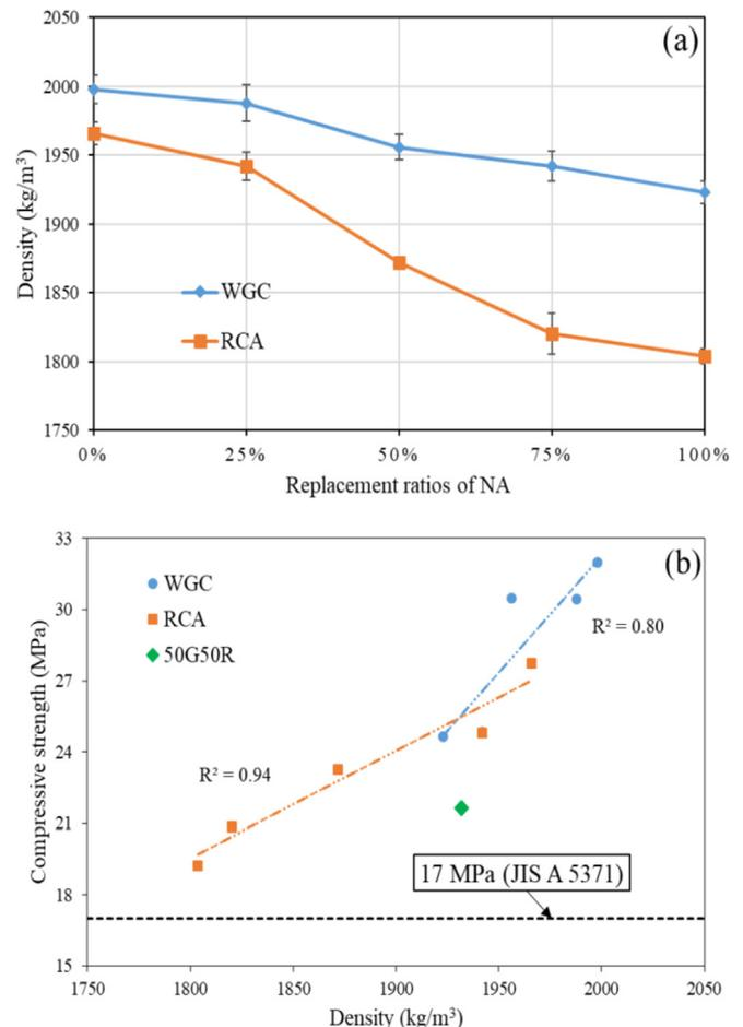
Fig. 6. Density of PCs prepared with WGC or RCA (a) and the correlation between compressive strength and density (b).
