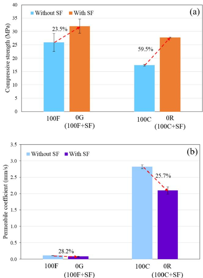
Fig. 4. Influence of aggregate sizes and SF on the compressive strength (a) and the permeability (b) of PCs.
