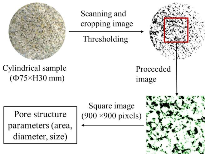
Fig. 3. Illustration of image analysis procedure employed.
