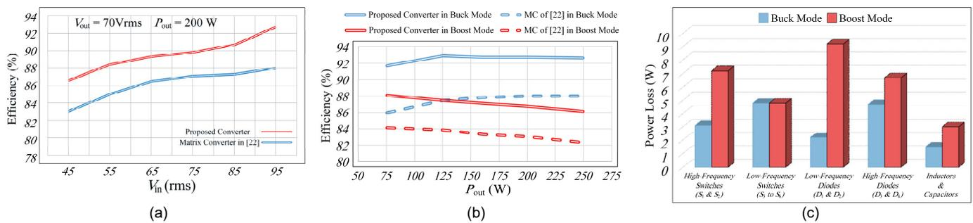
Fig. 9. Efficiency comparison of proposed converter (a) for various input voltage, (b) for various output power and (c) power loss distribution among components.
