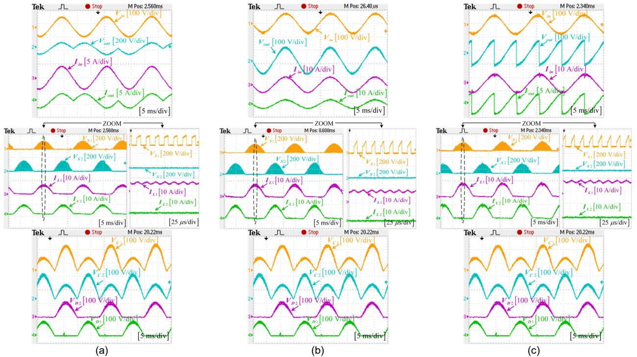
Fig. 8. Boost operation mode waveforms: input and output waveforms, blocked voltages by  $S_1$  and  $S_2$ , inductors currents, voltages across capacitors and inversed voltages across diodes  $D_1$  and  $D_2$  with output frequency of (a) 30Hz, (b) 60Hz, and (c) 120Hz.
