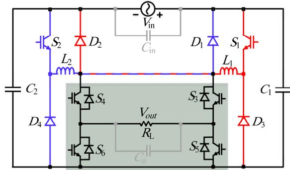
Fig. 2. Proposed single-phase buck-boost variable-frequency AC-AC converter.
