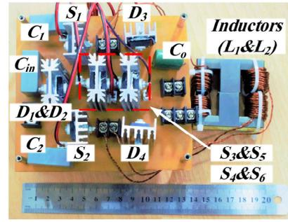
Fig. 6. Prototype of 200-W laboratory test rig.
