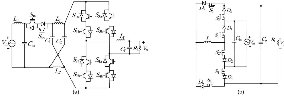
Fig. 1. Single-phase matrix converters with (a) the Z-source network of [21], and (b) six switch of [22].
