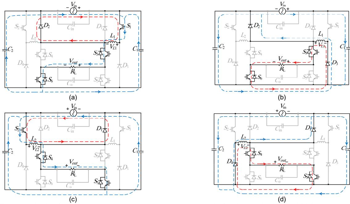
Fig. 4. Equivalent circuits of the proposed converter during input voltage positive half cycle in modes (a) I, and (b) II, and its negative half cycle in modes (c) I, and (d) II to generate 60Hz output voltage waveform.
