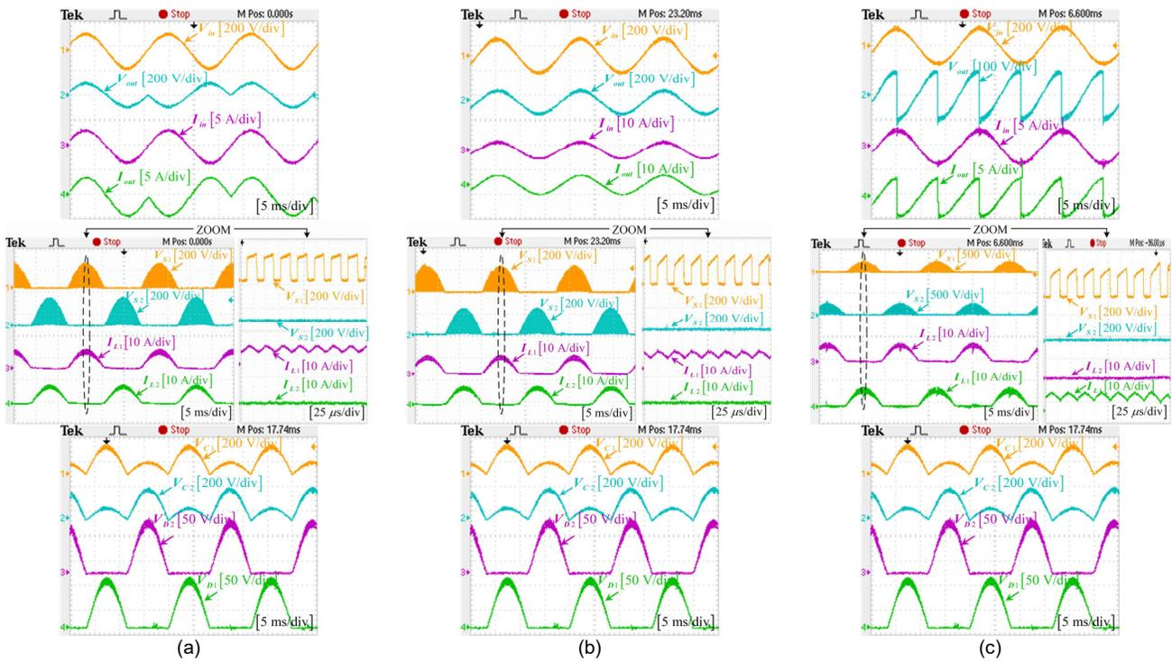
Fig. 7. Buck operation mode waveforms: input and output waveforms, blocked voltages by  $S_1$  and  $S_2$ , inductors currents, voltages across capacitors and inversed voltages across diodes  $D_1$  and  $D_2$  with output frequency of (a) 30Hz, (b) 60Hz, and (c) 120Hz.
