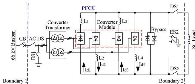
Fig. 2. The topology of ITER PF converter unit.
