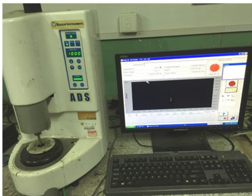
Fig. 5. Dynamic shear rheometer.
