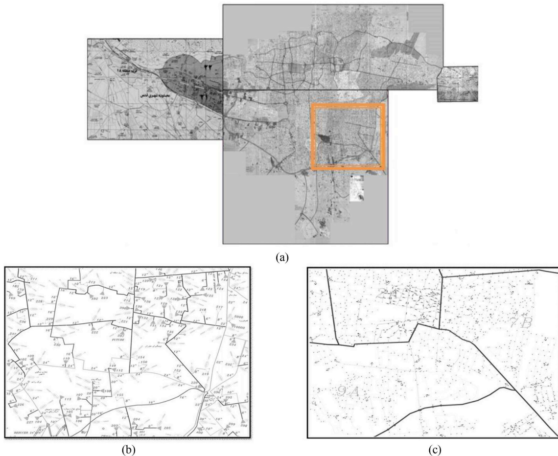
Fig. 6. (a) Selected area for performance assessment in liquefaction, (b) Network of high pressure gas pipelines, and (c) Network of medium pressure gas pipelines.
