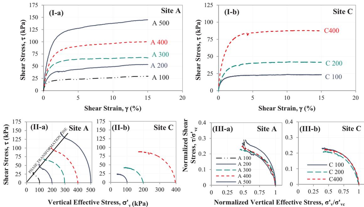
Fig. 3. Constant-volume monotonic DSS test results on relatively undisturbed specimens of natural silt retrieved from the Site A (data from [65]) and Site C (data from [66]) at normally consolidated stress state at varying confining stress levels: (I) shear stress-strain; (II) effective stress path; and (III) normalized effective stress path.
