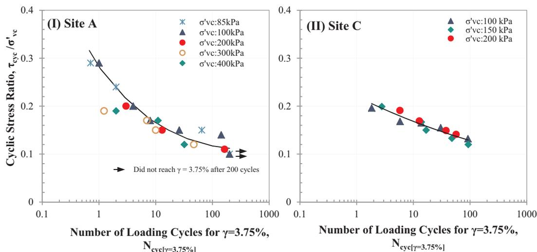
Fig. 4. Cyclic Stress Ratio (CSR) versus number of loading cycles required to reach  $\gamma = 3.75\%$  in constant-volume cyclic DSS tests on silts from (I) Site A (after [65]) and (II) Site C (after [20]).
