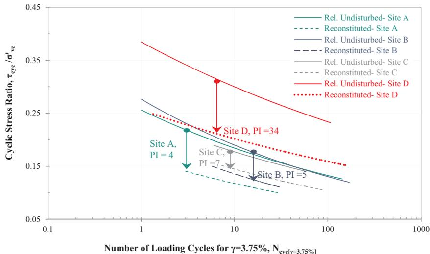
Fig. 19. CSR versus Number of loading cycles to reach  $\gamma = 3.75\%$  curves from constant-volume cyclic DSS tests on fine-grained material indicating the reduction of cyclic shear resistance of reconstituted specimen with respect to relatively undisturbed specimen from subject sites (after [20,70]).
