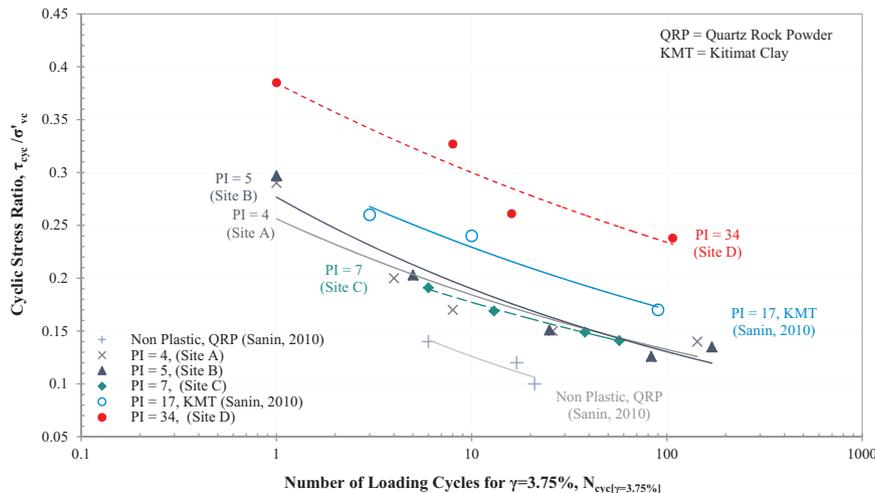
Fig. 15. CSR versus Number of loading cycles to reach  $\gamma = 3.75\%$  curves from constant-volume cyclic DSS tests on fine-grained materials with different plasticity (after [61,68]).
