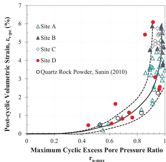
Fig. 20. Characteristics of post-cyclic volumetric strain ( $\epsilon_{v-pc}$ ) versus maximum cyclic pore-water pressure ratio ( $r_{u-max}$ ) during cyclic DSS loading from specimens from Site A, B, C and D, overlain with Quartz Rock Powder (QRP) (data from [19,20]).
