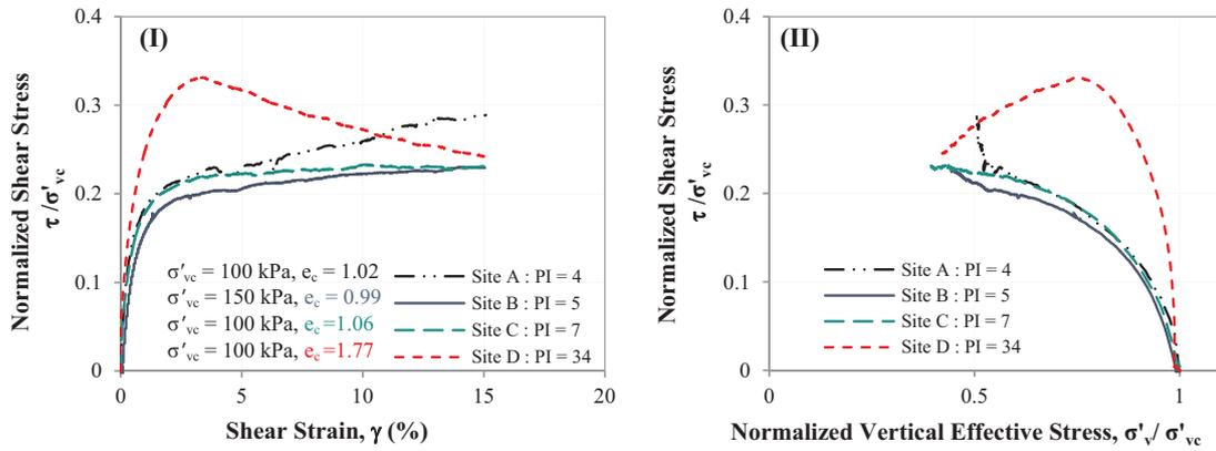
Fig. 14. (I) Normalized shear stress-strain response and (II) normalized stress path response of constant-volume monotonic DSS tests on undisturbed specimens of normally consolidated natural silt with different plasticity indices from Site A, B, C, and D (after [19,20]).
