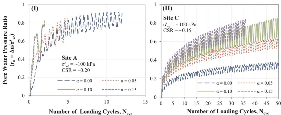
Fig. 11. Excess pore-water pressure development at different initial static shear values and constant CSR values for tested undisturbed specimens: (I) Site A (after [19]); and (II) Site C (after [67]).
