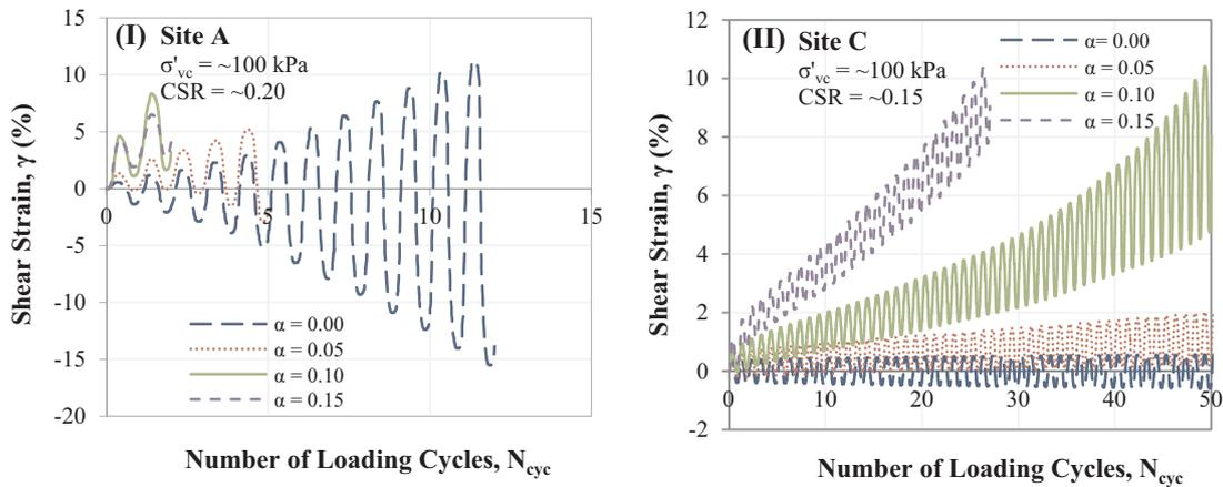
Fig. 12. Accumulation of shear strain at different initial static shear values and constant CSR values for tested undisturbed specimens: (I) Site A (after [19]); and (II) Site C (after [67]).
