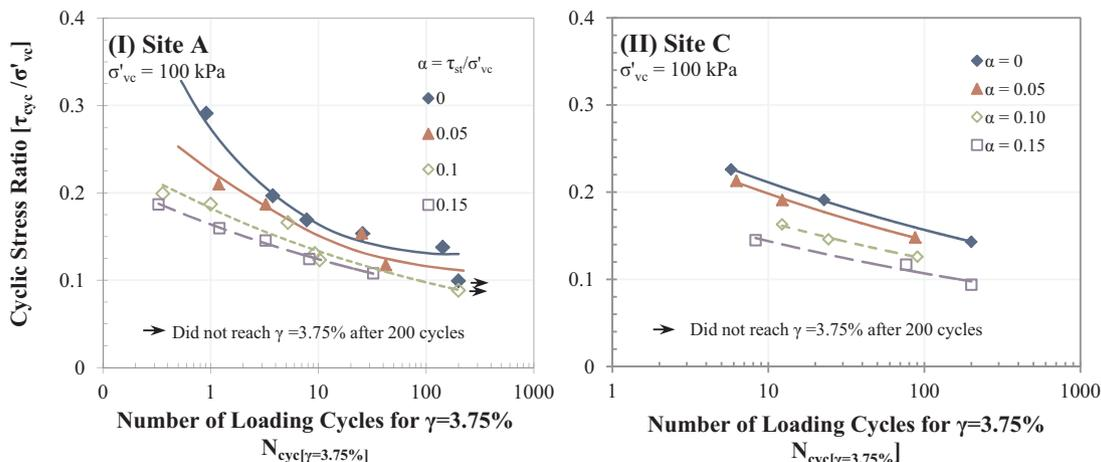
Fig. 13. CSR versus number of loading cycles required to reach  $\gamma = 3.75\%$  in from constant-volume cyclic DSS tests performed on undisturbed silt specimens at varying initial static shear bias: (I) Site A (after [19]); and (II) Site C (after [67]).
