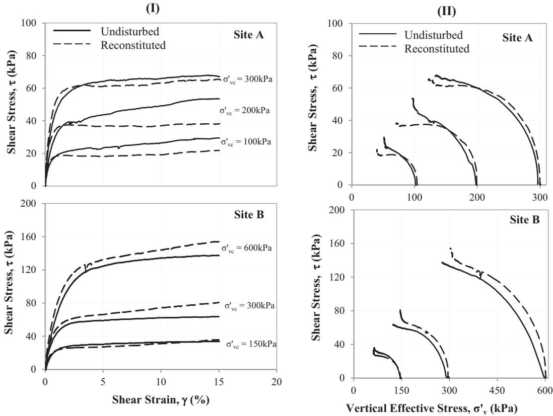
Fig. 16. The results from constant-volume monotonic DSS tests on undisturbed and reconstituted specimens prepared from Site A and B. (I) Shear stress-strain response; (II) Stress path response (after [19,69]).
