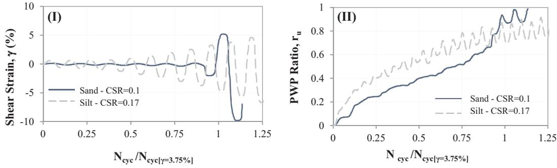
Fig. 2. (I) Typical strain accumulation and (II) pore-water pressure (PWP) development without static shear bias for loose Fraser River sand (data from [22]) and low-plastic undisturbed Fraser River silt (data from [19]).
