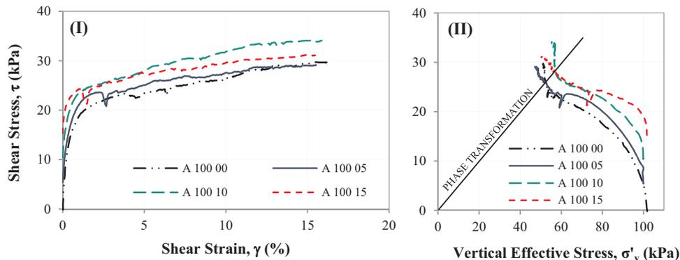
Fig. 9. (I) Shear stress-strain response and (II) stress path response of constant-volume monotonic DSS tests on relatively undisturbed specimens from Site A at varying initial static shear bias ( $\alpha$ ):  $\sigma'_{vc} = 100$  kPa;  $\alpha = 0, 0.05, 0.10, 0.15$  (after [19]).
