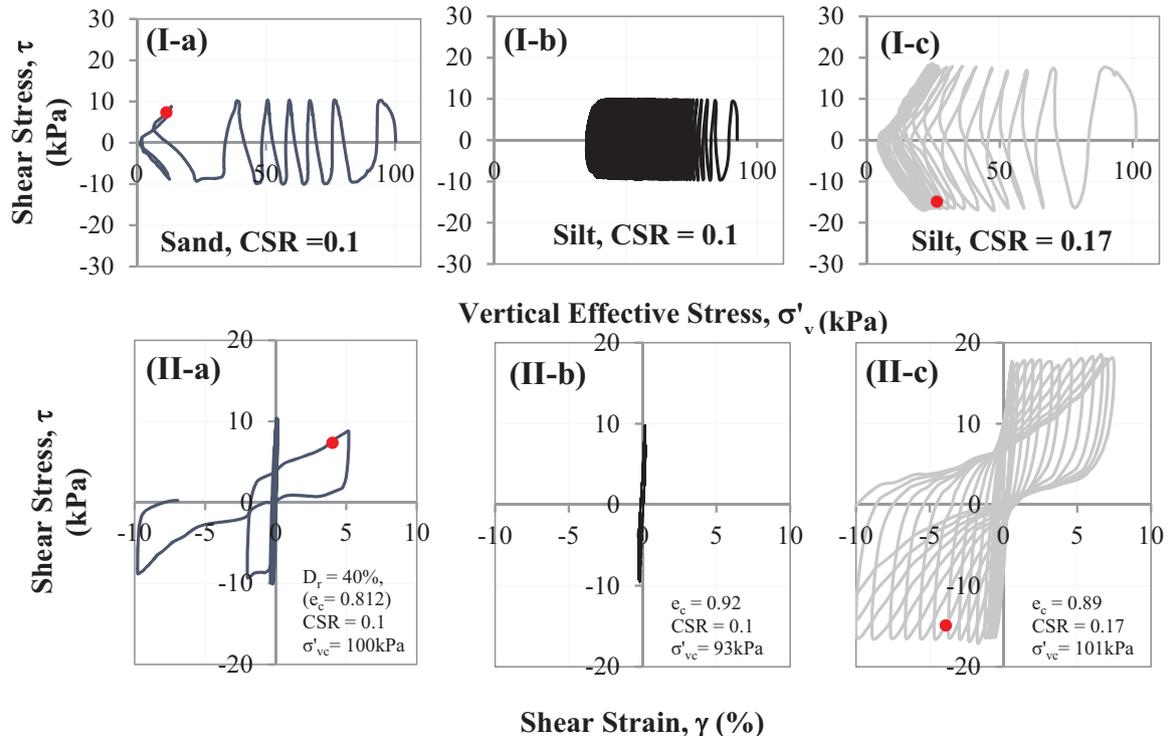
Fig. 1. Typical response without static shear bias - Loose Fraser River sand: (I-a) effective stress path; (II-a) shear stress-strain response (data from [21]); Low-plastic undisturbed Fraser River silt: (I-b and I-c) effective stress path; (II-b and II-c) shear stress-strain (data from [19]). Note: Red dot indicates the onset of  $\gamma = 3.75\%$ .
