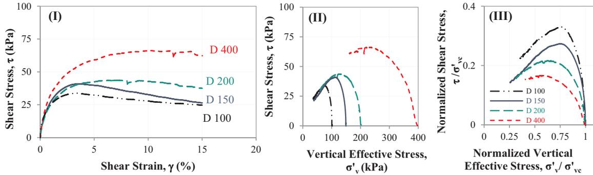
Fig. 5. Constant-volume monotonic DSS test results on relatively undisturbed specimens of natural silt retrieved from the Site D at normally consolidated stress state at varying confining stress levels: (I) shear stress-strain; (II) effective stress path; and (III) normalized effective stress path (after [66]).
