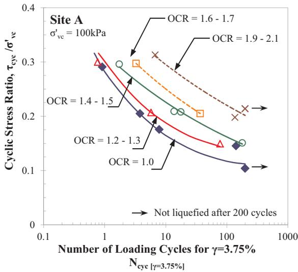
Fig. 8. Cyclic shear loading response: CSR versus  $N_{cyc[\gamma=3.75\%]}$  for different OCRs on specimens from Site A (after [24]).
