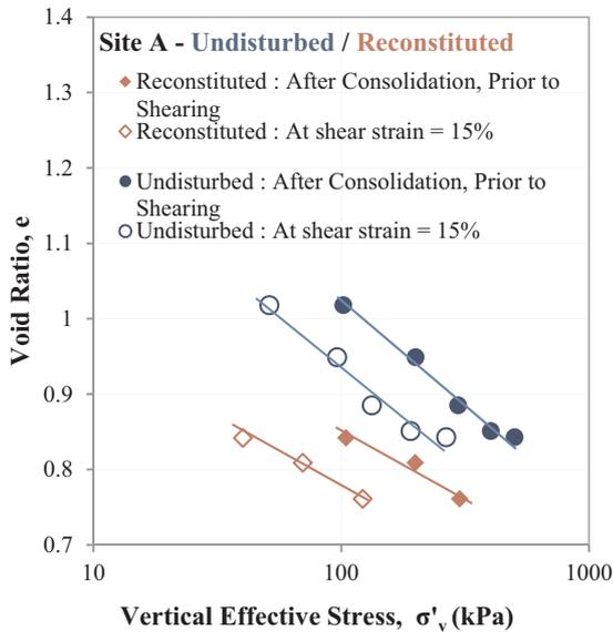
Fig. 17.  $e$ - $\log \sigma'_v$  relationships for undisturbed and reconstituted specimens of Fraser River silt after initial consolidation (prior to shearing) compared with those after reaching 15% shear strain in monotonic direct simple shear (after [19]).
