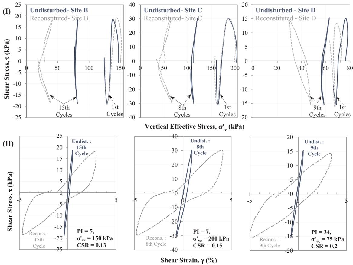
Fig. 18. Comparison of (I) stress path and (II) shear stress-strain curves of selected loading cycles during constant-volume cyclic DSS test on undisturbed and reconstituted specimen under similar normally consolidated  $\sigma'_{vc}$  and CSR from Site B [PI = 5], C [PI = 7], and D [PI = 34] (after [20]).
