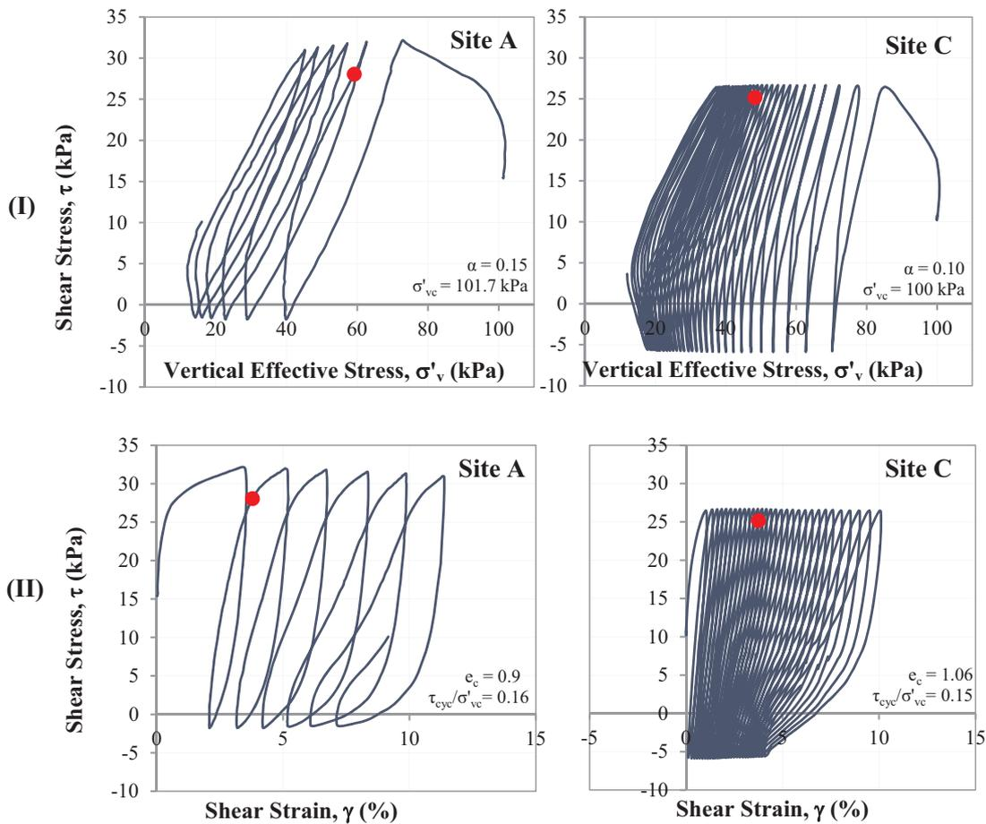
Fig. 10. (I) Typical stress path and (II) stress-strain response of constant-volume cyclic DSS tests with initial static shear bias on relatively undisturbed specimens from Site A (after [19]) and C (after [67]). Note: Red dot indicates the onset of  $\gamma = 3.75\%$ .
