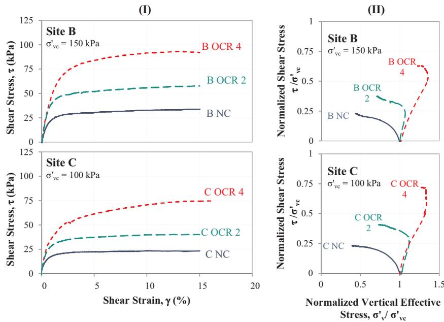
Fig. 7. (I) Shear stress-strain response and (II) normalized stress path response of constant-volume monotonic DSS tests on relatively undisturbed specimens from Site B and C, at confining stress states of NC, OCR 2 and OCR 4 (after [66]).
