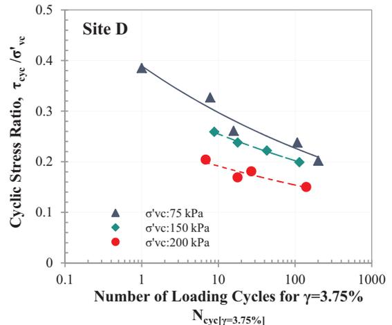
Fig. 6. CSR versus number of loading cycles required to reach  $\gamma = 3.75\%$  in constant-volume cyclic DSS tests on silts from Site D (after [30]).
