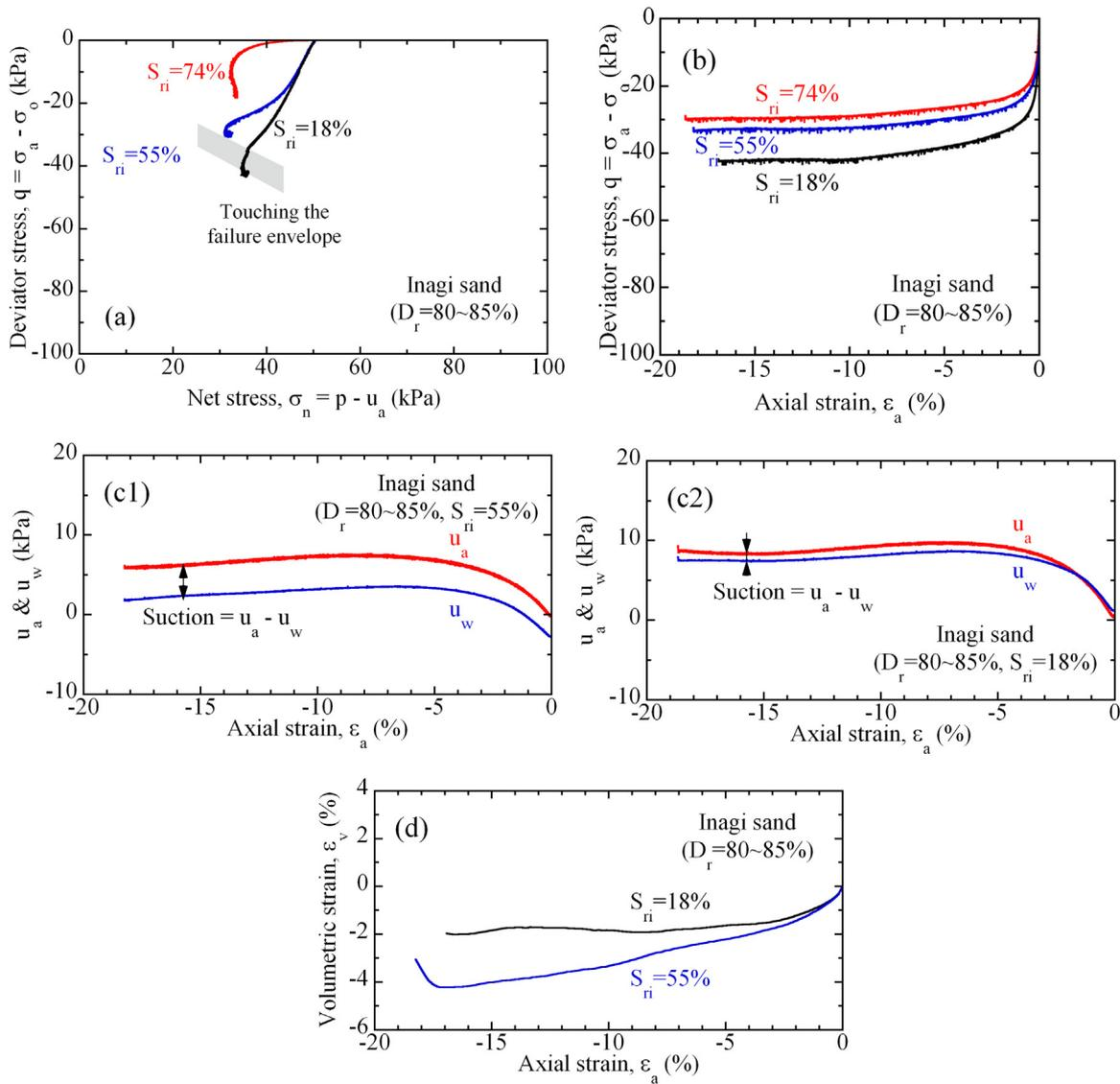
Fig. 12. Results of unsaturated undrained triaxial extension tests, (a) net stress  $\sigma_n = p - u_a$  – deviator stress  $q = \sigma_a - \sigma_o$ , (b) axial strain  $\epsilon_a$  – deviator stress  $q$ , (c) axial strain  $\epsilon_a$  – pore air and pore water pressures,  $u_a$  &  $u_w$ , (d) axial strain  $\epsilon_a$  – volumetric strain  $\epsilon_v$ , (Inagi sand,  $D_r = 80\text{--}90\%$ ).
