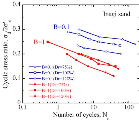
Fig. 8. Plots of cyclic stress ratio  $\sigma_d/(2\sigma'_o)$  against number of cycles  $N_c$  in partially saturated undrained cyclic triaxial tests, (Inagi sand).
