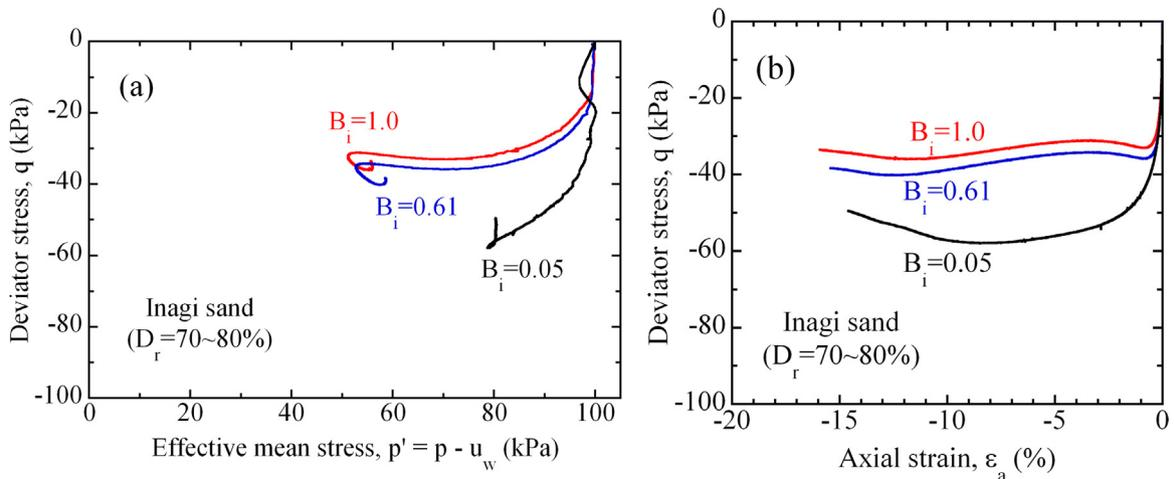
Fig. 6. Results of partially saturated undrained triaxial extension tests, (a) effective mean stress  $p'$  – deviator stress  $q$ , (b) axial strain  $\epsilon_a$  – deviator stress  $q$ , (Inagi sand,  $D_r = 70\sim 80\%$ ).
