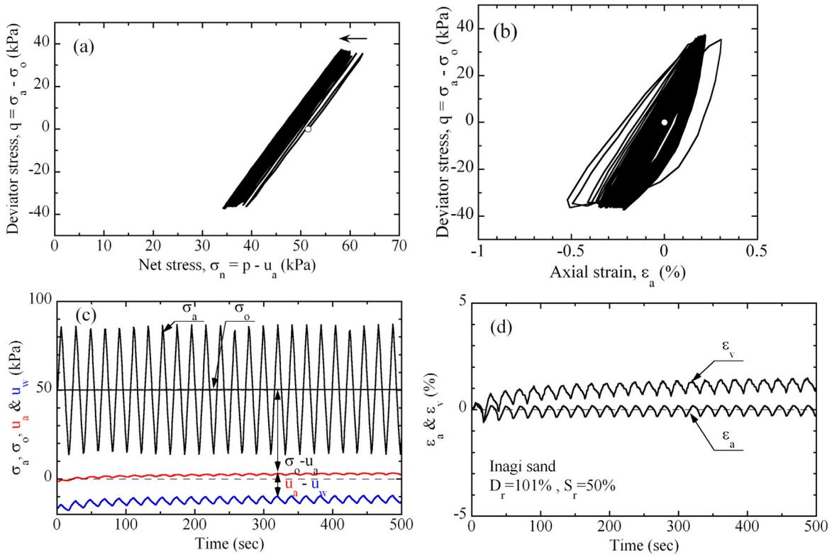
Fig. 15. Results of unsaturated undrained cyclic triaxial tests, (a) net stress  $\sigma_n = p - u_a$  – deviator stress  $q = \sigma_a - \sigma_o$ , (b) axial strain  $\epsilon_a$  – deviator stress  $q$ , (c) time - axial stress  $\sigma_a$ , confining stress  $\sigma_o$  and pore air pressure  $u_a$ , (d) time - axial strain  $\epsilon_a$  and volumetric strain  $\epsilon_v$ , (Inagi sand,  $D_r = 101\%$ ,  $S_r = 50\%$ ).
