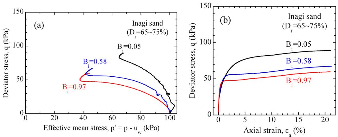
Fig. 5. Results of partially saturated undrained triaxial compression tests, (a) effective mean stress  $p'$  – deviator stress  $q$ , (b) axial strain  $\epsilon_a$  – deviator stress  $q$ , (Inagi sand,  $D_r = 65\sim 75\%$ ).
