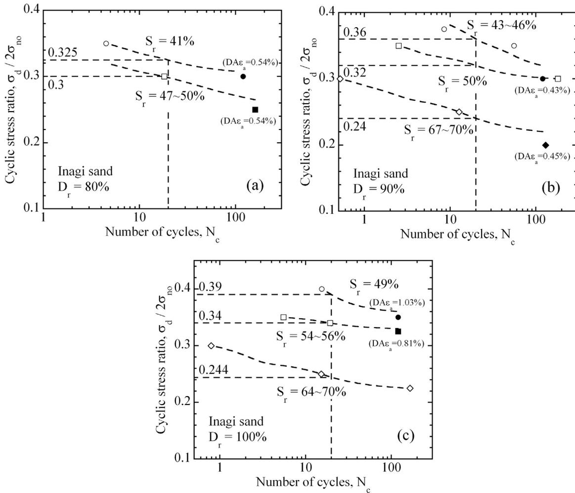
Fig. 16. Plots of cyclic stress ratio  $\sigma_d/2\sigma_{no}$  against number of cycles, (Inagi sand), (a)  $D_r = 80\%$ , (b)  $D_r = 90\%$ , (c)  $D_r = 100\%$ .
