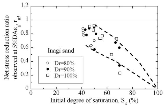
Fig. 18. Plots of net stress reduction ratio observed at  $5\%DA\varepsilon_a$ ,  $r_{ns}$ , against  $S_{ri}$ , (Inagi sand).
