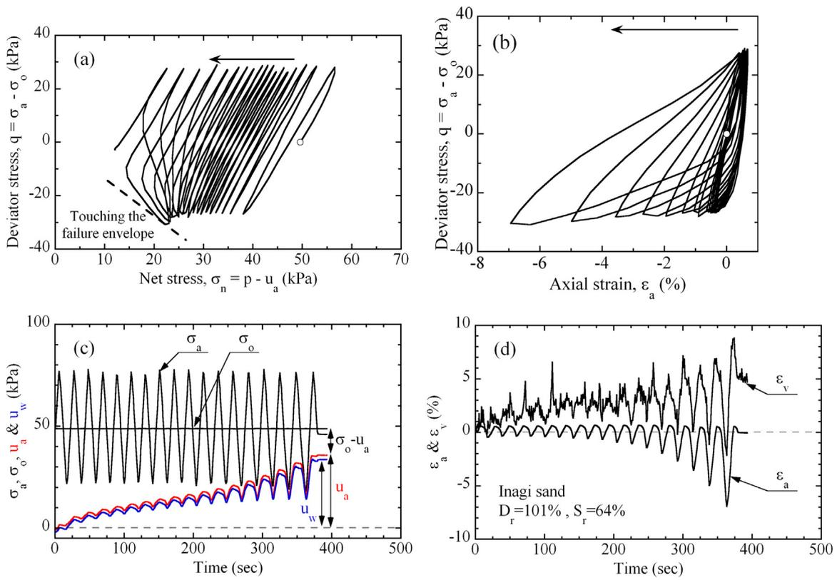
Fig. 14. Results of unsaturated undrained cyclic triaxial tests, (a) net stress  $\sigma_n = p - u_a$  – deviator stress  $q = \sigma_a - \sigma_o$ , (b) axial strain  $\epsilon_a$  – deviator stress  $q$ , (c) time - axial stress  $\sigma_a$ , confining stress  $\sigma_o$  and pore air pressure  $u_a$ , (d) time - axial strain  $\epsilon_a$  and volumetric strain  $\epsilon_v$ , (Inagi sand,  $D_r = 101\%$ ,  $S_r = 64\%$ ).
