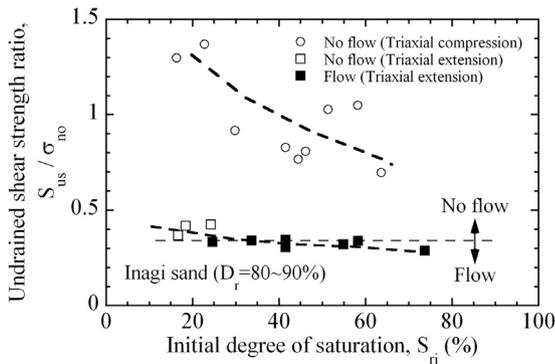
Fig. 13. Plots of unsaturated undrained shear strength ratio  $S_{us}/\sigma'_{o}$  against initial degree of saturation  $S_{ri}$ , (Inagi sand,  $D_r = 80\text{--}90\%$ ).
