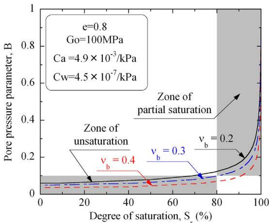
Fig. 2. Relation between degree of saturation  $S_r$  and coefficient of pore water pressure  $B$ .
