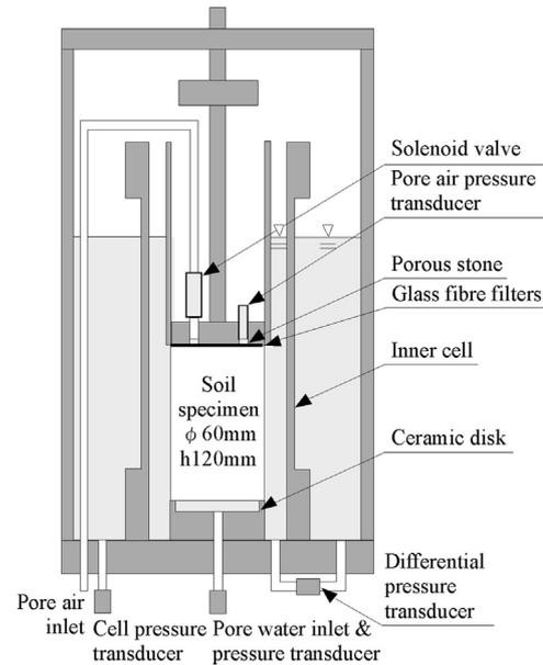
Fig. 10. Experimental setup of unsaturated triaxial tests.
