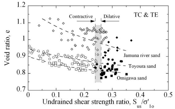
Fig. 3. Plots of saturated undrained shear strength ratio  $S_{us}/\sigma'_{1_0}$  against void ratio  $e$  (data after Tsukamoto et al., 2009).
