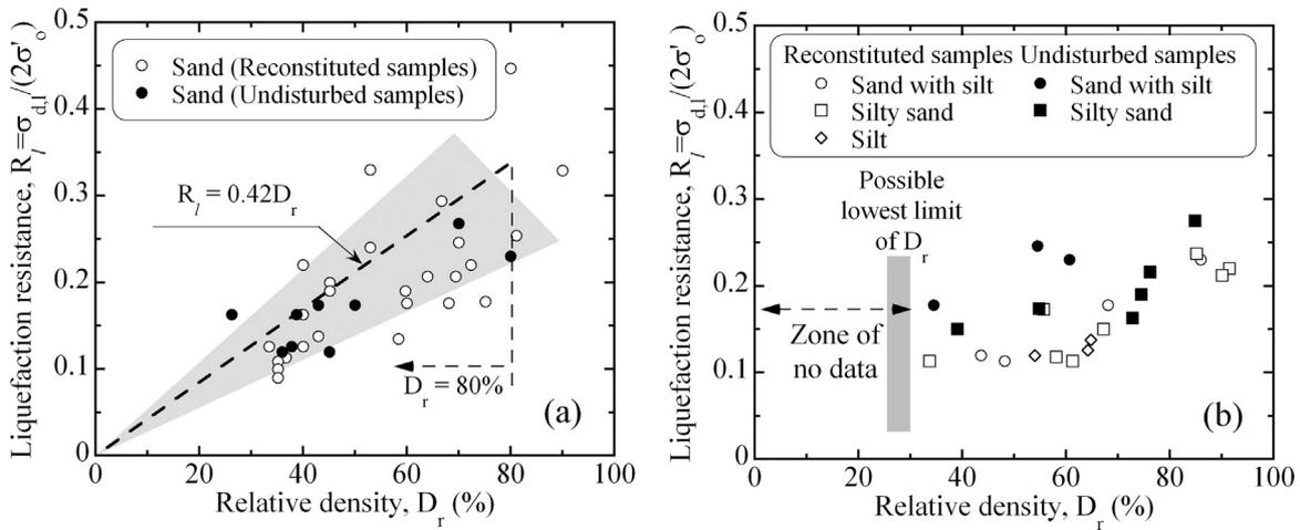
Fig. 4. Plots of saturated liquefaction resistance  $R_l$  against relative density  $D_r$ , (a) clean sand, (b) silty sand.
