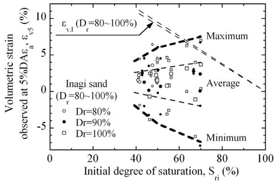
Fig. 19. Plots of volumetric strain observed at 5%DAε<sub>a</sub>, ε<sub>v5</sub>, against S<sub>r,i</sub>, (Inagi sand).
