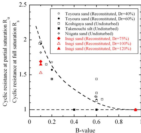
Fig. 9. Plots of ratios of partially saturated cyclic resistance  $R_u$  to fully saturated cyclic resistance  $R_s$  against  $B$ -value.
