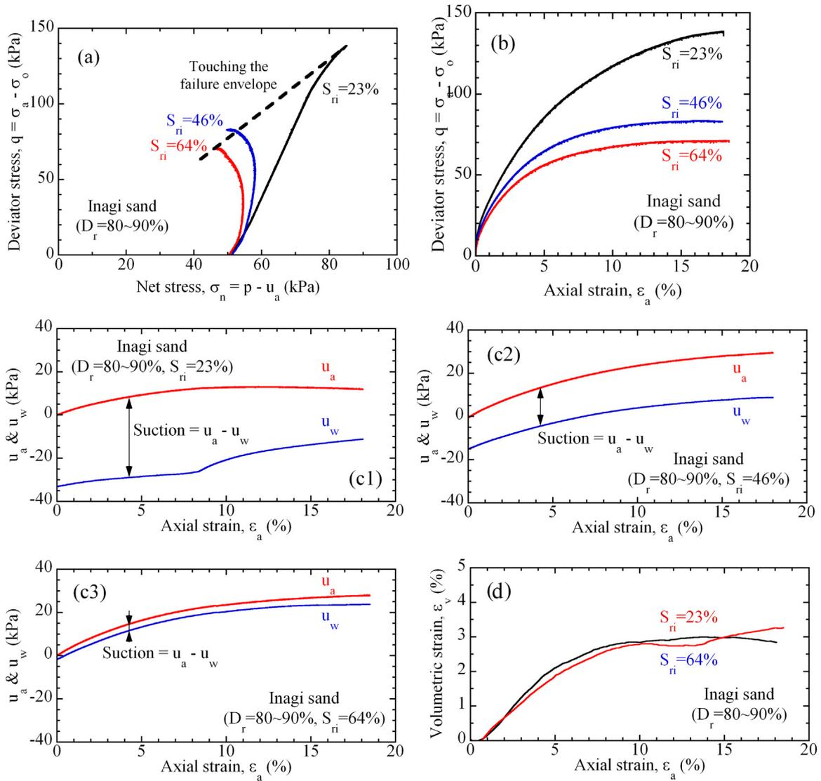
Fig. 11. Results of unsaturated undrained triaxial compression tests, (a) net stress  $\sigma_n = p - u_a$  - deviator stress  $q = \sigma_a - \sigma_o$ , (b) axial strain  $\epsilon_a$  - deviator stress  $q$ , (c) axial strain  $\epsilon_a$  - pore air and pore water pressures,  $u_a$  &  $u_w$ , (d) axial strain  $\epsilon_a$  - volumetric strain  $\epsilon_v$ , (Inagi sand,  $D_r = 80\text{--}90\%$ ).
