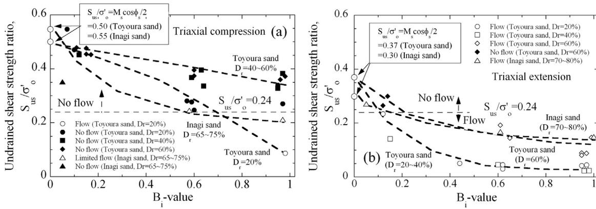
Fig. 7. Plots of partially saturated undrained shear strength ratio  $S_{us}/\sigma'_o$  against initial  $B_i$ -value, (Toyoura clean sand & Inagi silty sand), (a) triaxial compression, (b) triaxial extension.
