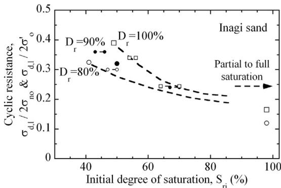
Fig. 17. Plots of unsaturated cyclic resistance  $\sigma_{d,l}/2\sigma_{no}$  and saturated liquefaction resistance  $\sigma_{d,l}/2\sigma'_o$  against  $S_{ri}$ , (Inagi sand).
