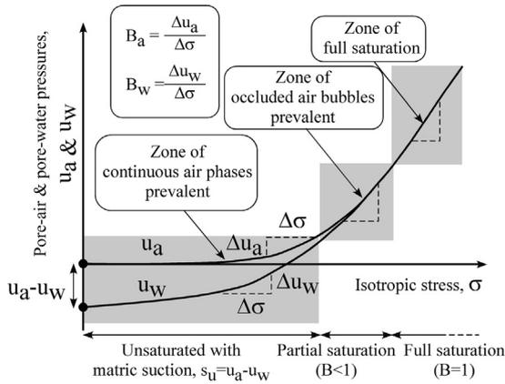
Fig. 1. Confining stress – pore pressure relations in soils.
