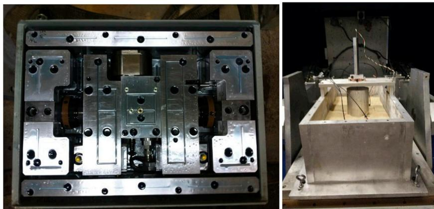
Fig. 1. CWRU electro-hydraulic shaker (L) and test platform (R).
