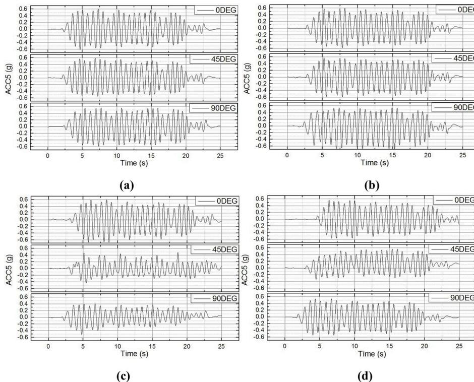
Fig. 11. Time histories of acceleration recorded by ACC5(a) Toyoura sand, dry (b) Nevada sand, Dry(c) Toyoura sand, saturated (d) Nevada sand, saturated.
