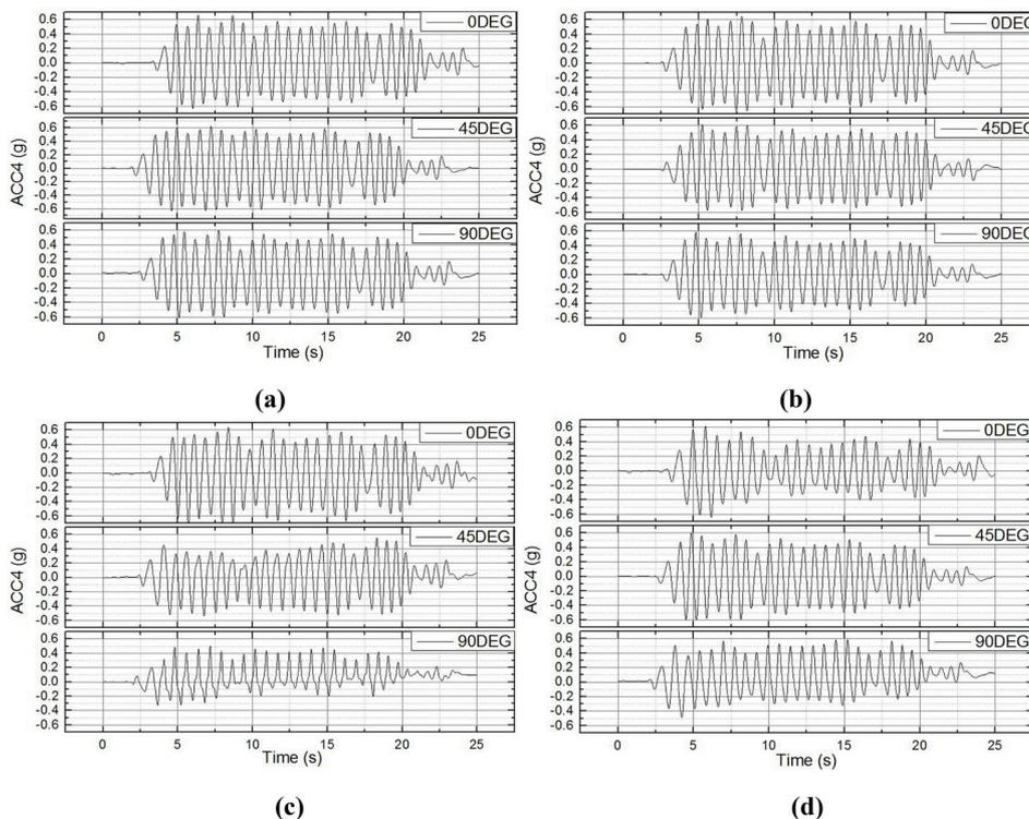
Fig. 9. Time histories of acceleration recorded by ACC4. (a) Toyoura sand, dry (b) Nevada sand, Dry(c) Toyoura sand, saturated (d) Nevada sand, saturated.
