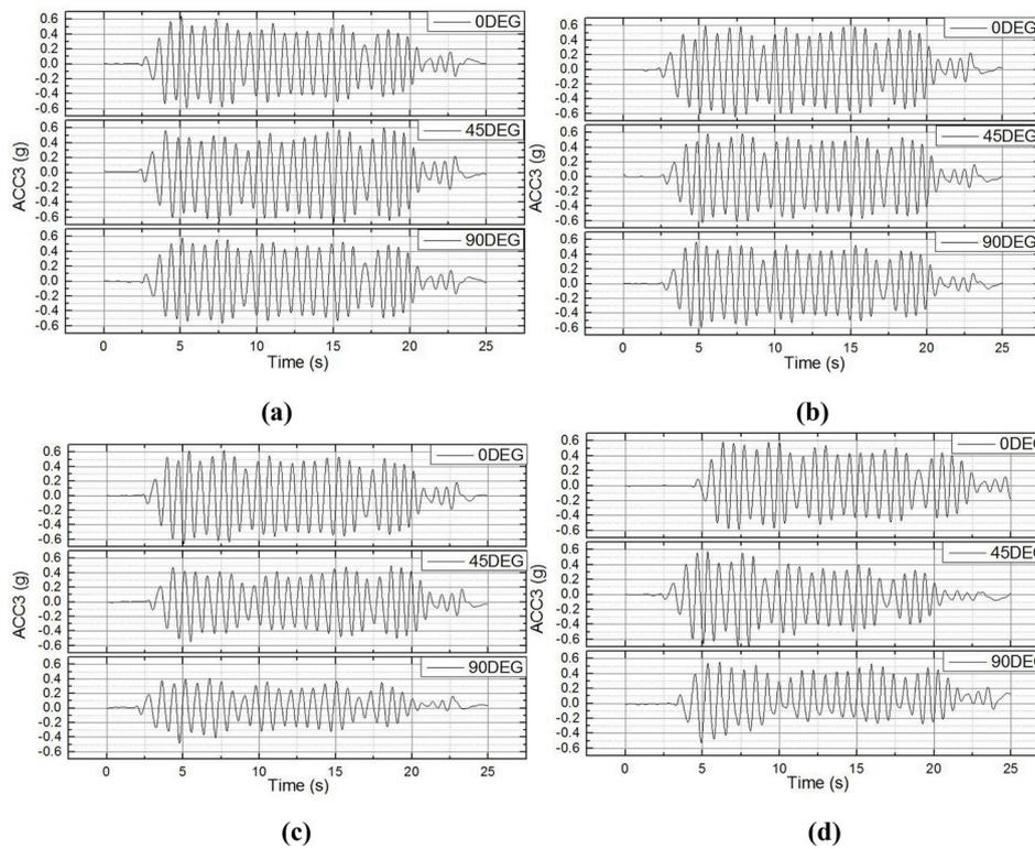
Fig. 10. Time histories of acceleration recorded by ACC3. (a) Toyoura sand, dry (b) Nevada sand, Dry(c) Toyoura sand, saturated (d) Nevada sand, saturated.
