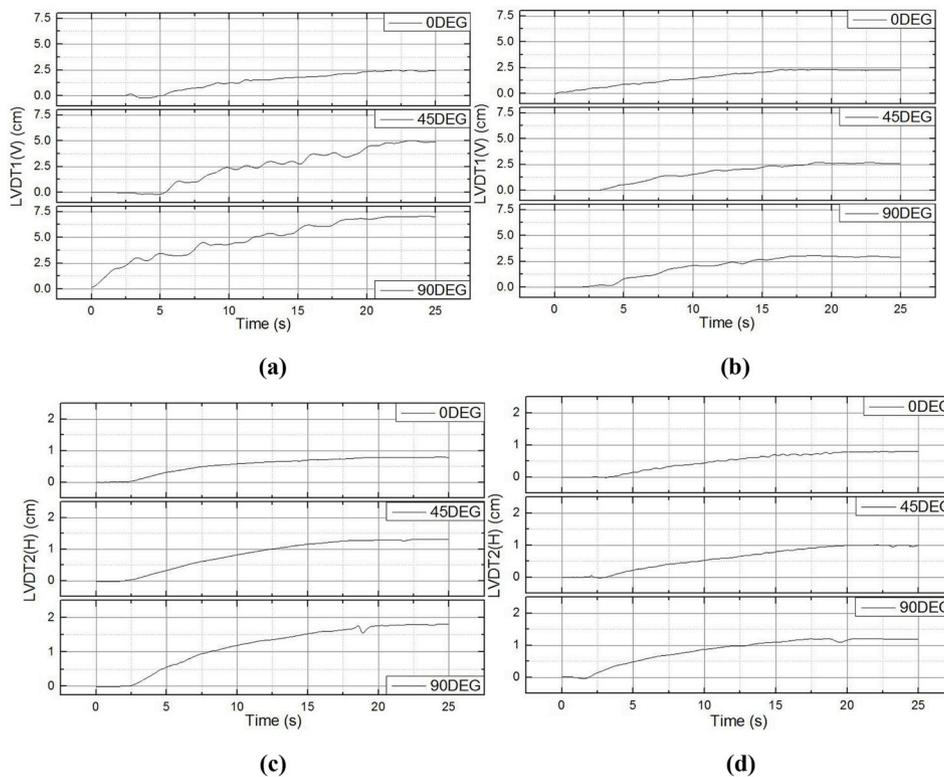
Fig. 14. Time histories recorded by LVDTs in dry condition. (a) Toyoura S and, vertical displacement (b) Nevada S and, vertical Displacement. (c) Toyoura S and, horizontal displacement (d) Nevada S and, horizontal displacement.
