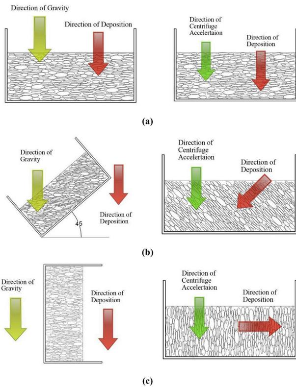
Fig. 5. (a) Model preparation with 0 degree deposition Angle(b) model preparation with 45 degree deposition Angle(c) model preparation with 90 degree deposition angle.
