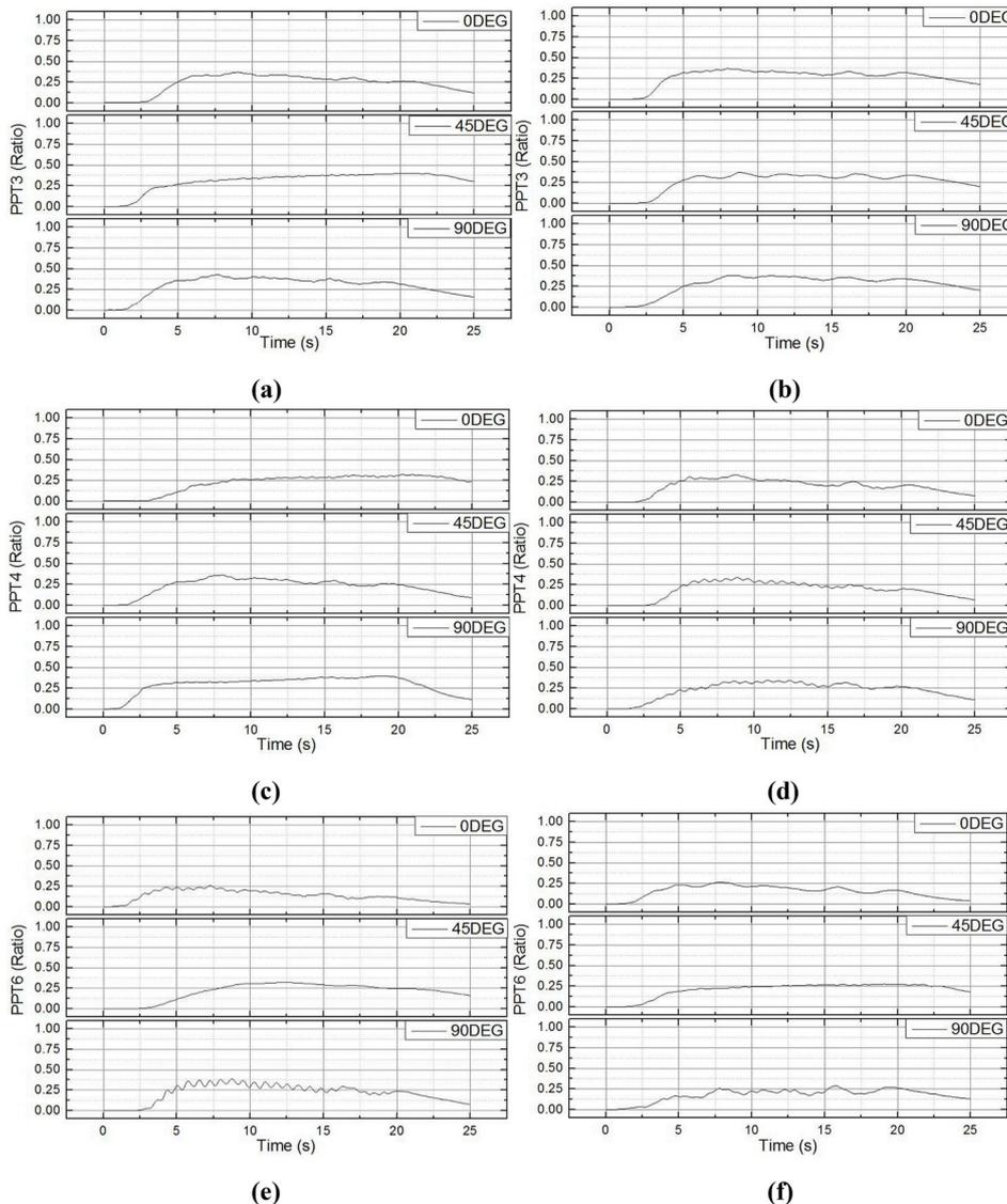
**Fig. 12.** Time histories recorded by pore pressure transducers. (a) Toyoura, saturated condition (PPT3) (b) Nevada, saturated condition (PPT3)(c) Toyoura, saturated condition (PPT4) (d) Nevada, saturated condition (PPT4)(e) Toyoura, saturated condition (PPT6) (f) Nevada, saturated condition (PPT6).
