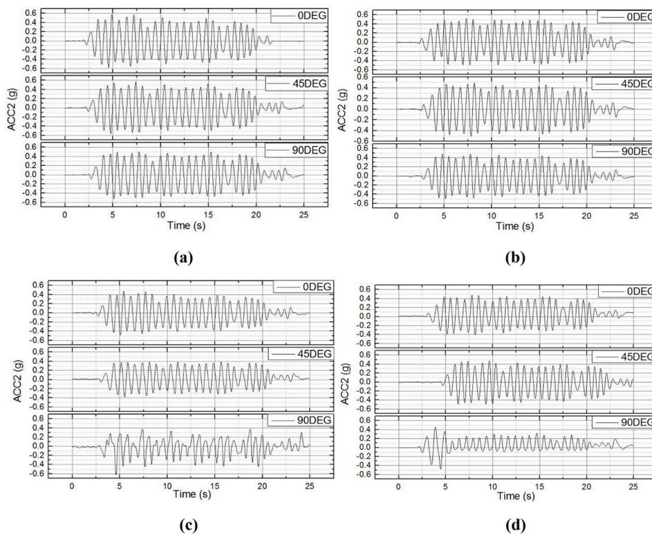
Fig. 8. Time histories of acceleration recorded by ACC2. (a) Toyoura sand, dry (b) Nevada sand, Dry(c) Toyoura sand, saturated (d) Nevada sand, saturated.
