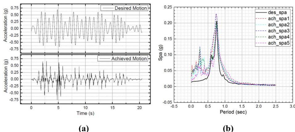
**Fig. 7.** (a) Comparison between achieved motion and design motion in time History. (b) comparison between achieved motion and design motion in spectral acceleration.
