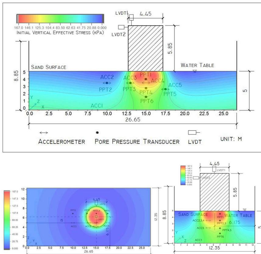
Fig. 6. Cross-sectional view of the centrifuge model.
