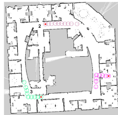
Fig. 11. Trajectories used for pose tracking tests. The starting points of the trajectories are indicated by red points. (For interpretation of the references to color in this figure legend, the reader is referred to the web version of this article.)
