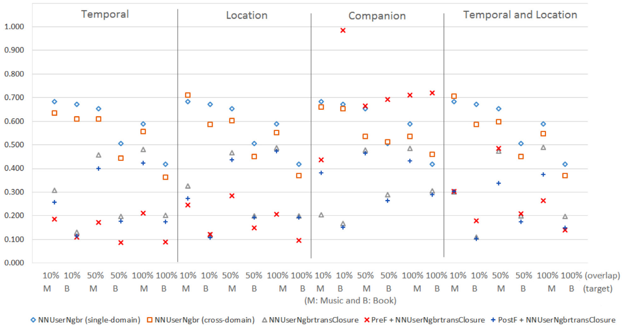
Fig. 7. MAE performance for the algorithms by varying target domain (book and music), contextual dimension and user overlap levels.
