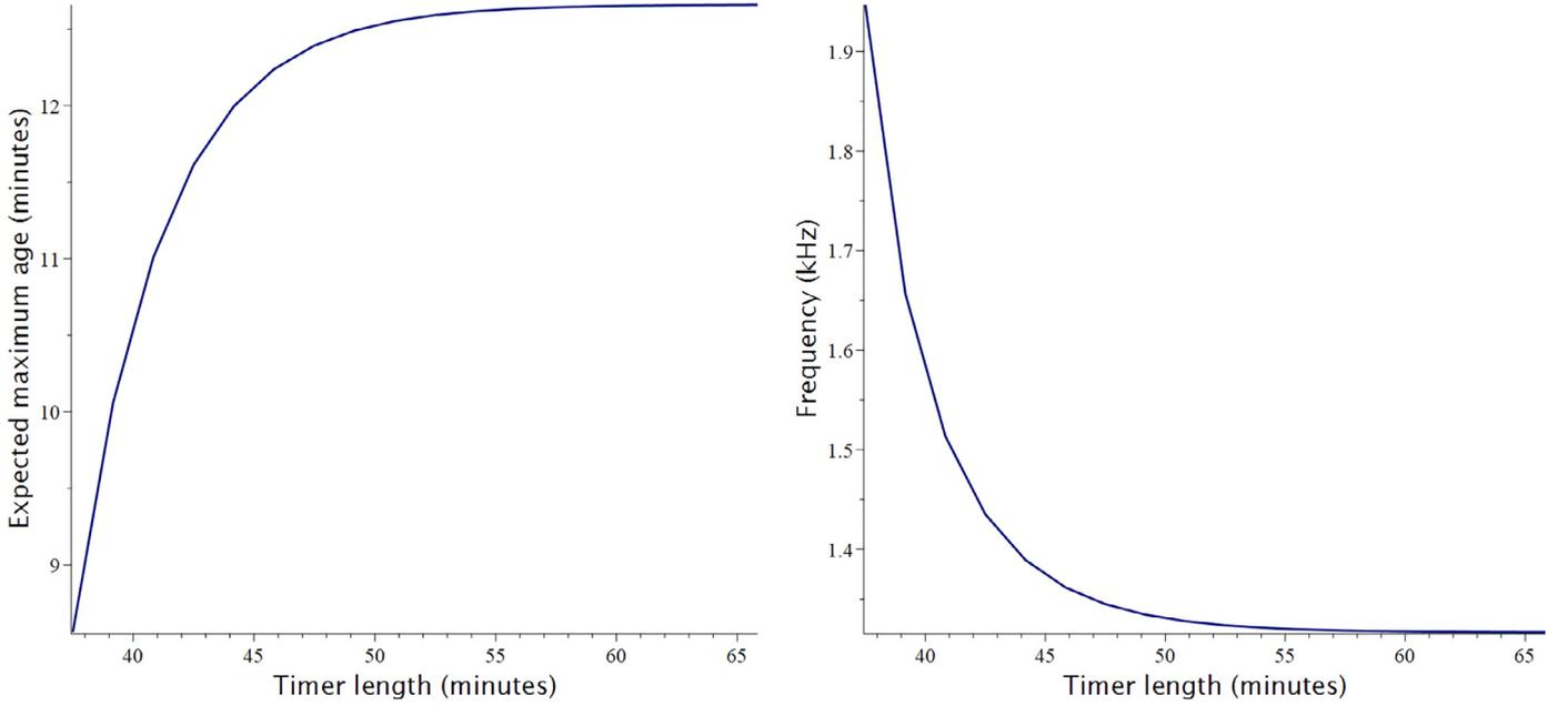
Fig. 7. Maximum age of data and frequency of backup with change in timer length.  $\lambda = 0.07$ , slot length = 5 second,  $\alpha_i = \frac{i}{30}$ , and  $l = 20$ .
