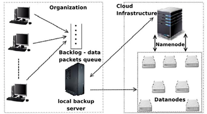
Fig. 1. Components of data backup mechanism.
