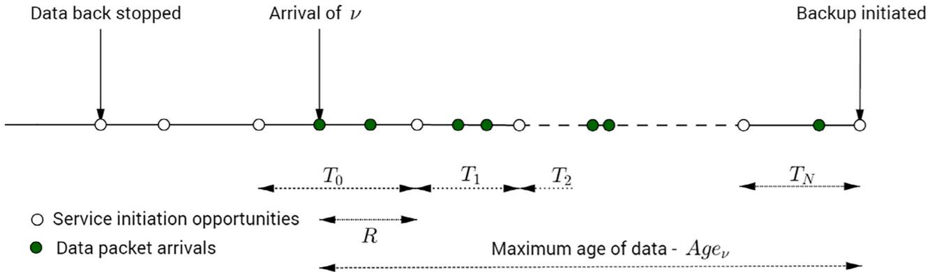
Fig. 3. Illustration of delay of packet  $\nu$ .
