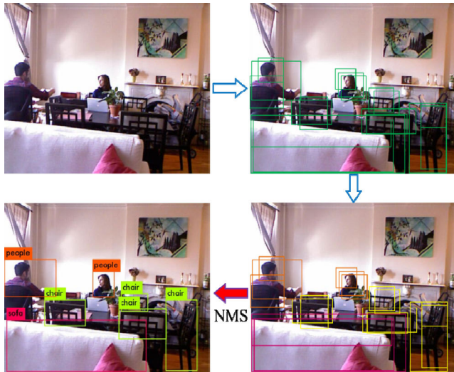
FIGURE 1. The diagram of the non-maximum suppression algorithm.
