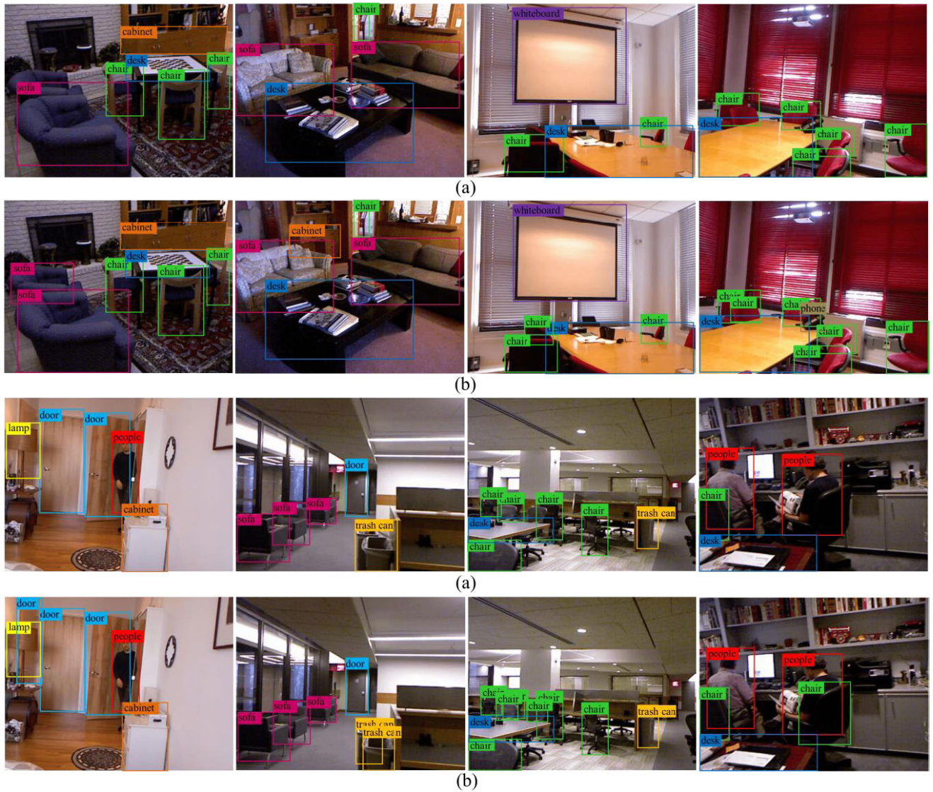
FIGURE 6. Some of the RGB-D object detection results based on the NYU Depth V2 dataset for (a), the traditional NMS algorithm and (b), the Depth Fusion NMS algorithm.
