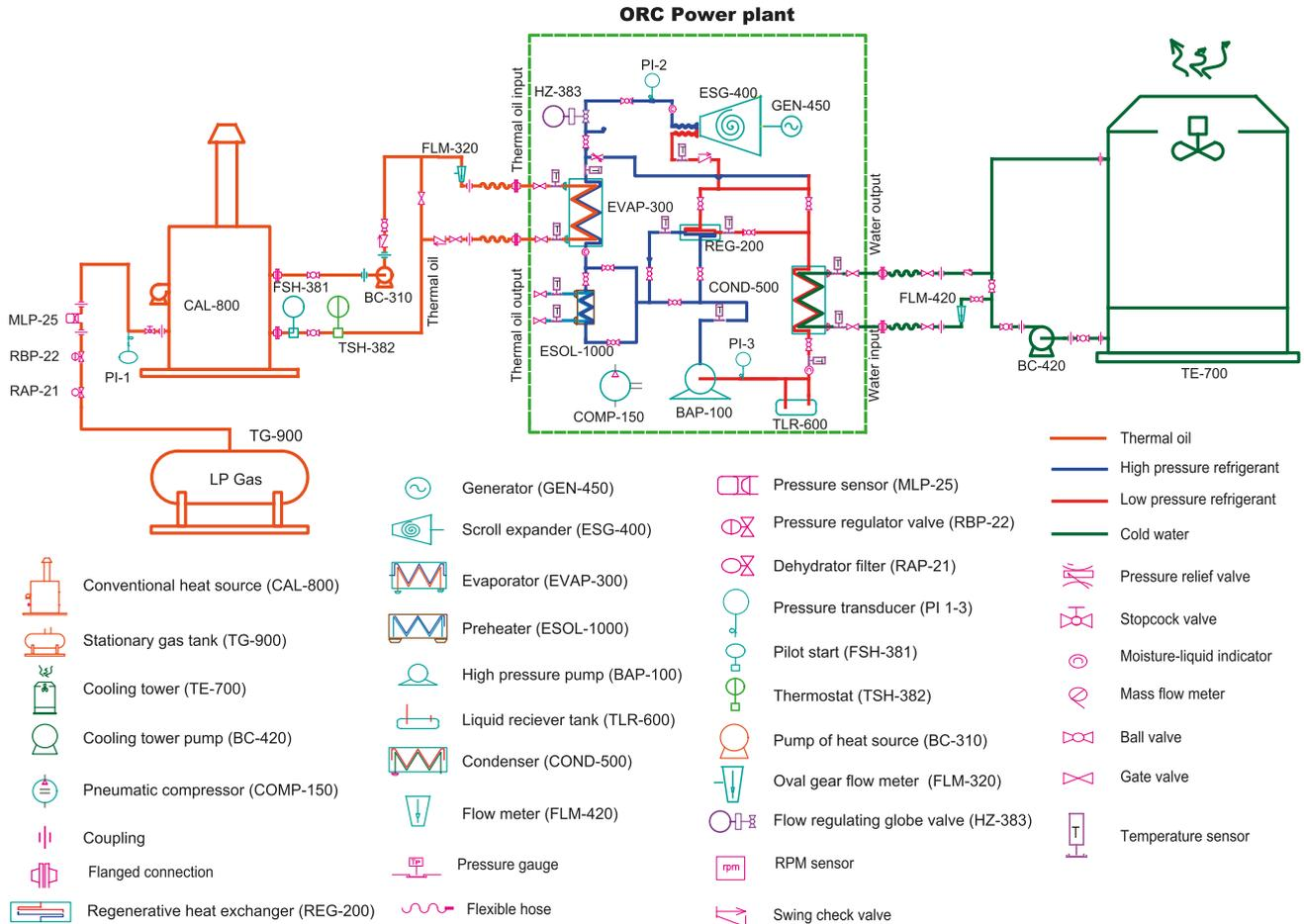
FIGURE 2. Instrumentation diagram and piping (P&ID) of ORC.
