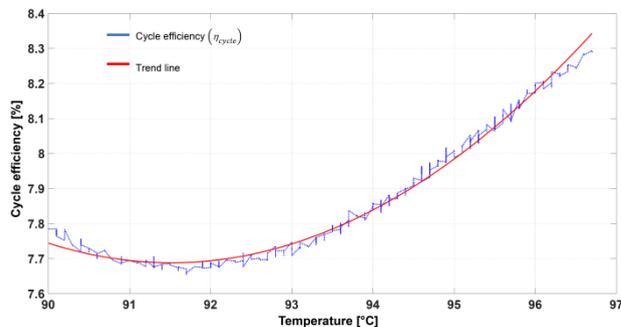
FIGURE 6. Relationship of the cycle efficiency and expander working flow temperature.
