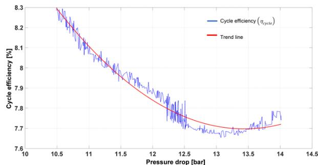
FIGURE 7. The relationship between fluid pressure drop and cycle efficiency in the system.
