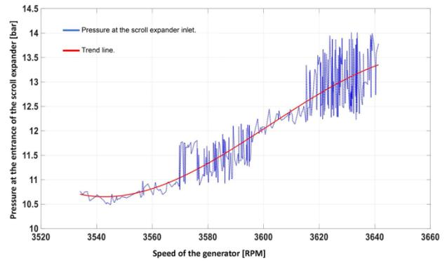
FIGURE 5. The relationship between speed angle and scroll expander pressure.
