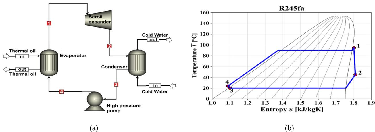
FIGURE 1. a) ORC plant schematic and b) the operation represented in Temperature-entropy (T-s) diagram for R245fa working fluid.
