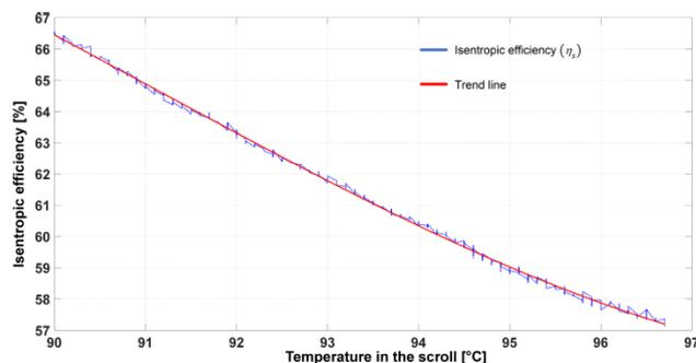
FIGURE 8. The relationship between inlet temperature the working fluid at the inlet of the scroll expander and isentropic efficiency of the scroll expander.
