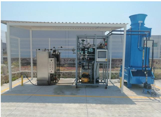
FIGURE 3. Electric energy generating ORC plant prototype.
