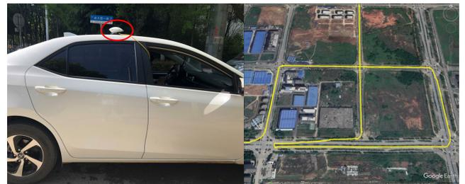
FIGURE 8. Observational environment and GNSS antenna in the car-driven experiment (trajectory of the car with yellow line).
