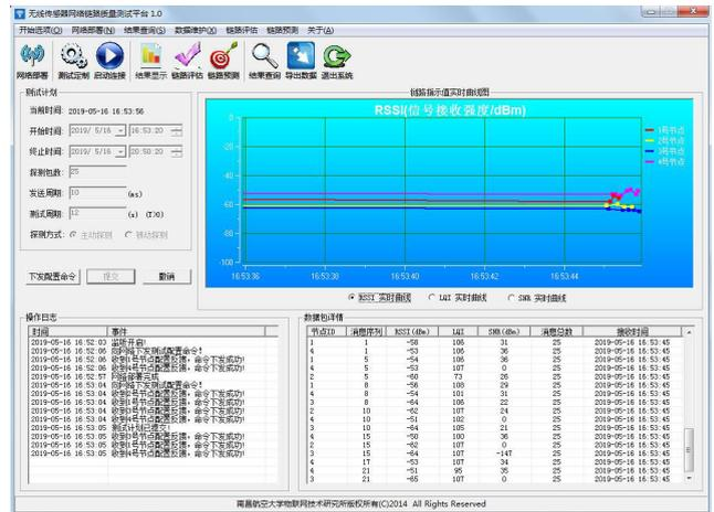
FIGURE 3. WSN Link Quality Testbed (WSNs-LQT).
