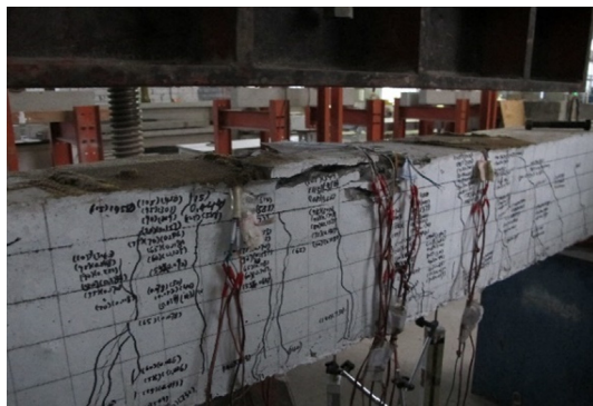
Fig. 6. Failure mode of beam L-1.
