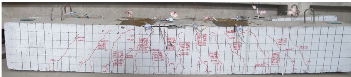
Fig. 7. Failure mode of beam L-2.
