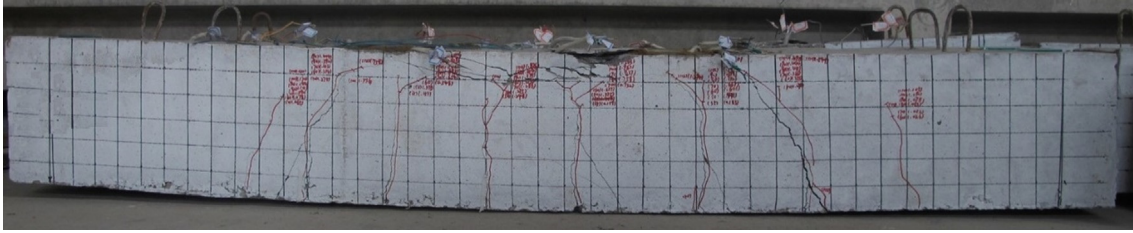
Fig. 10. Failure mode of beam L-5.
