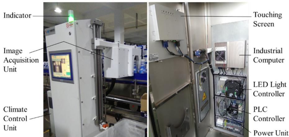
Fig. 2. The code inspection station installed in a beverage packaging line.
