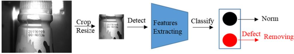
Fig. 12. Inspection process of the in-line inspection system.
