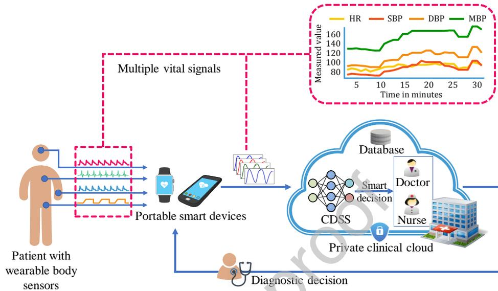
Figure 1: The typical architecture of remote healthcare systems. Portable smart devices collect multi biologicals of a patient with body sensors and sent these data to the server. The clinical institution can host the server in the Cloud or locally. A CDSS is used to do the smart prediction which supports the diagnosis from clinicians. If an abnormal event is detected, the system can notify the patient properly.
