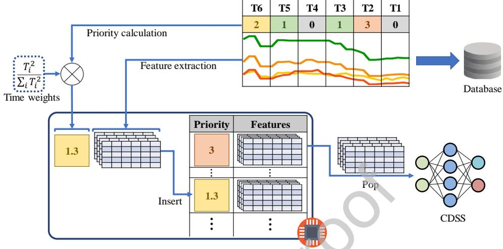
Figure 6: The workflow of the priority processor. The general priority of sequential TWDCs is calculated by TWDC priorities and the time weights. Based on the priority, the features of the whole TWDCs are inserted to the waiting list for predicting. Data with the highest priority in the list is processed by the CDSS.
