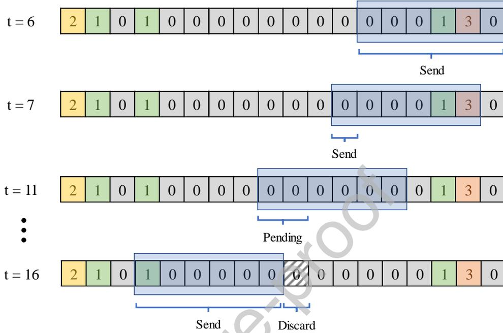
Figure 5: An example of data transmission. One new TWDC comes to the list as the increase of  $t$ . The blue buffer window includes all TWDCs processed by the system. In every  $t$ , the status of TWDCs are shown. In particular, pending of a TWDC means the system need to obtain more TWDCs to decide whether the TWDC should be sent or discarded.
