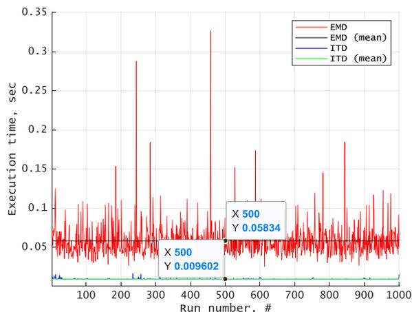
FIGURE 8. EMD vs ITD: runtime with averaging over 1000 measurements.
