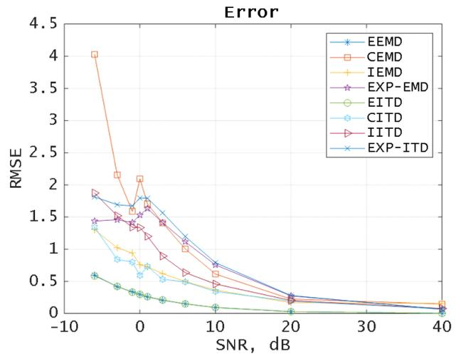
FIGURE 16. Comparison of various denoising algorithms for the “Blocks” signal.
