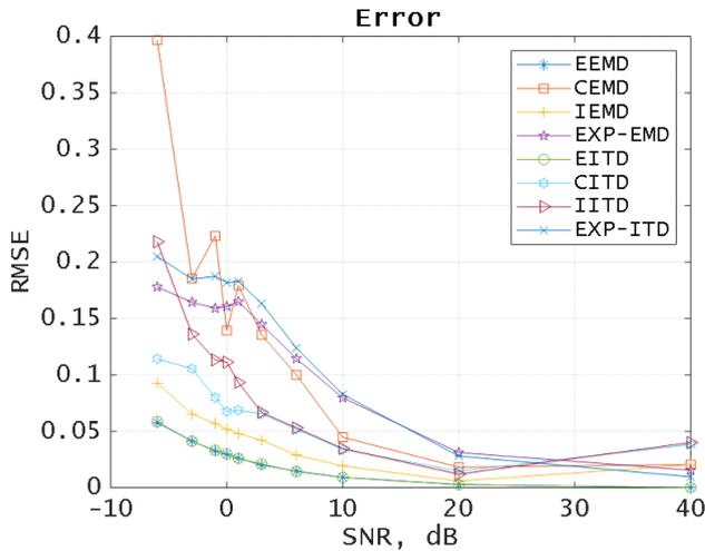
FIGURE 19. Comparison of various denoising algorithms for the "Doppler" signal.
