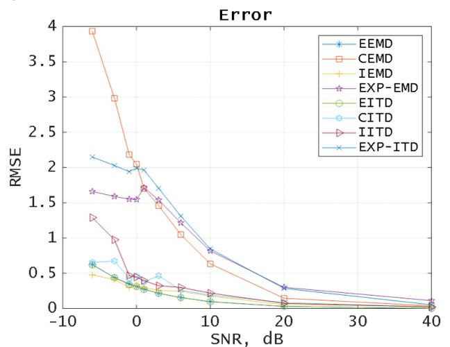
FIGURE 18. Comparison of various denoising algorithms for the “Heavy Sine” signal.
