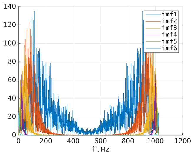
FIGURE 5. Filter bank based on EMD.
