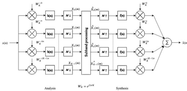
**FIGURE 2. Model of a DFT modulated filter bank based on full modulation.**
