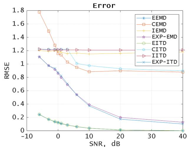
FIGURE 21. Comparison of various denoising algorithms for the "Mishmash" signal.
