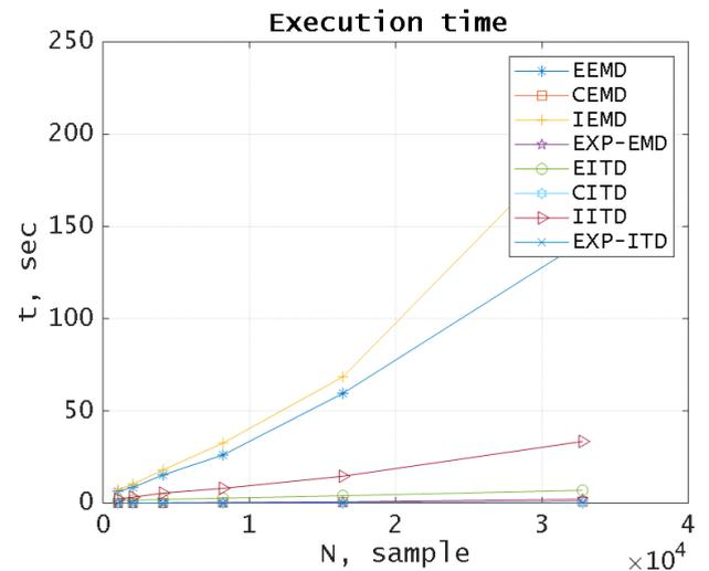
FIGURE 22. Comparison of computational complexity for various denoising algorithms.
