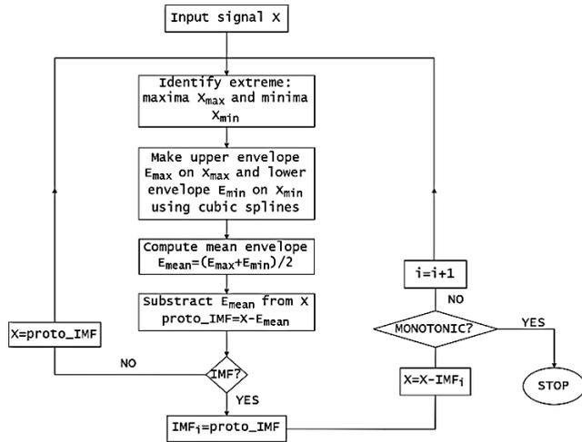
FIGURE 1. Block diagram of the EMD algorithm.
