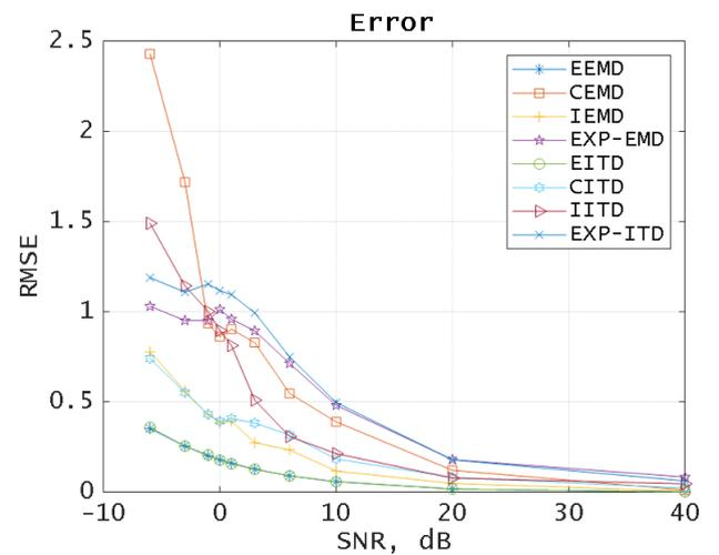
FIGURE 17. Comparison of various denoising algorithms for the “Bumps” signal.
