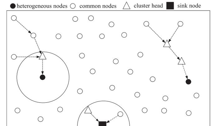
Fig. 3. Data transmission mode.
