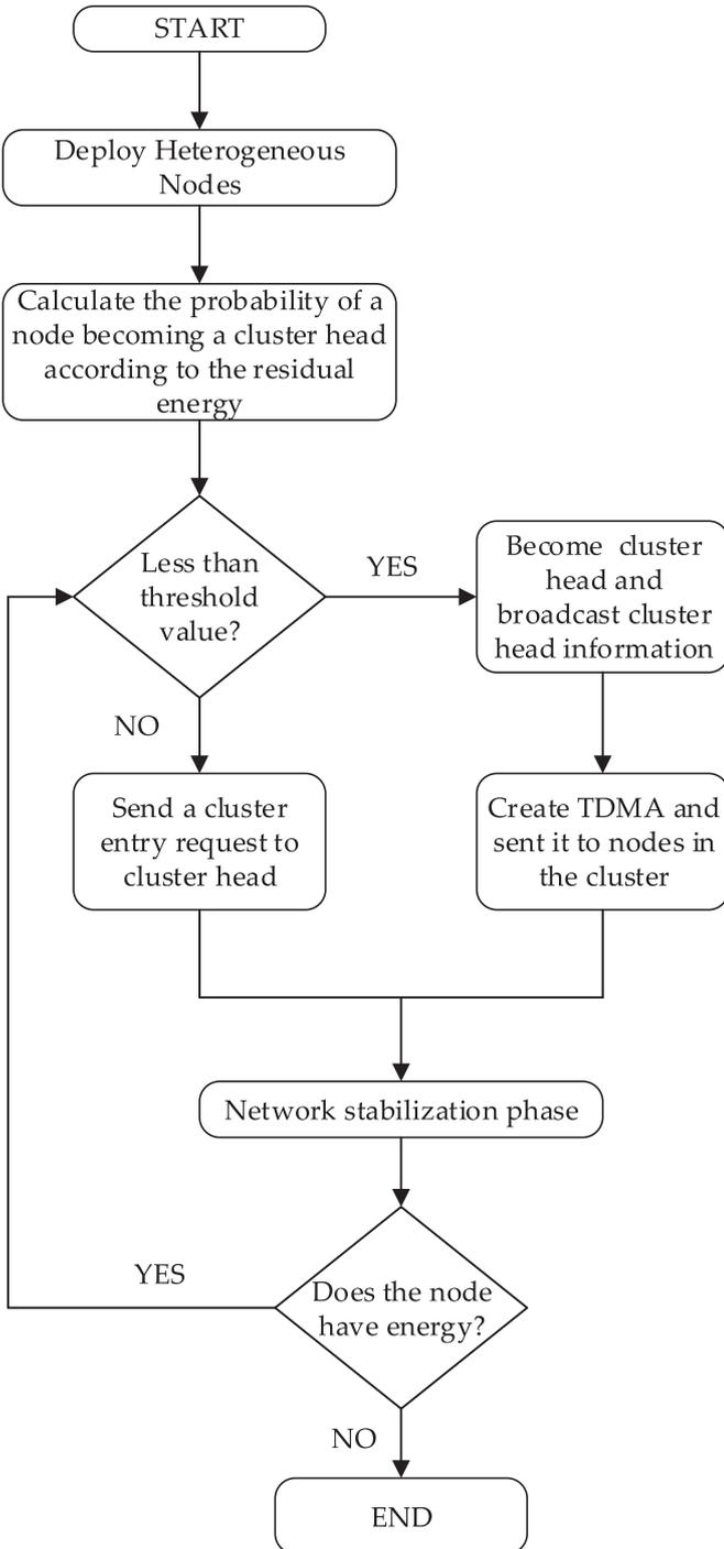
Fig. 2. The process of cluster head election.
