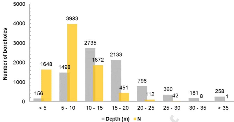
Figure 2. Statistical analysis of the depth of the boreholes and the number of SPT results per borehole.
