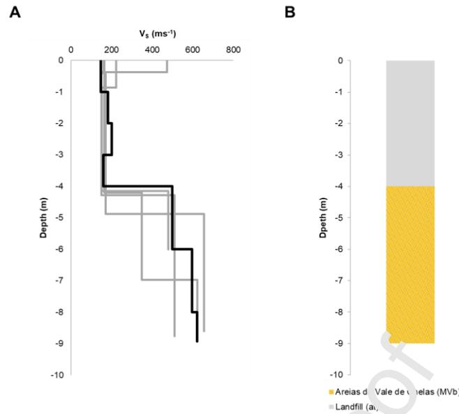
Figure 13.  $V_s$  profiles obtained from the analysis seismic profiles of surface waves for Musgueira site: A – obtained  $V_s$  profiles (in bold is the mean  $V_s$  profile); B – interpretative soil profile derived from the mean  $V_s$  profile.
