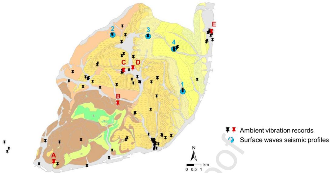
Figure 12. Location of the sites where ambient vibration records and surface waves seismic profiles were performed: A – Restelo; B – Campolide; C – Campo Grande; D – Campo Grande; E – Parque das Nações; 1 – Chelas; 2 – Quinta dos Alentejans; 3 – Musgueira; 4 – Encarnação.
