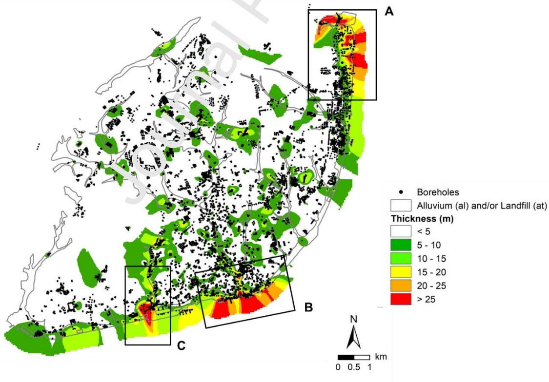
Figure 4. Distribution of surface formations (alluvium and landfill) in Lisbon, applying a data interpolation for thicknesses > 5 meters. A – Parque das Nações; B – Baixa; C – Alcântara.
