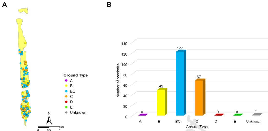
Figure 10. Areolas de Cabo Ruivo (MVIIb). A - Distribution of ground types on the geological formation (all classes considered); B - Histogram with the accounting of ground type, considering the new class BC.
