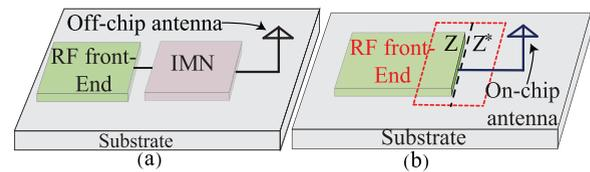
**FIGURE 19.** Comparison of off-chip and on-chip antennas w.r.t impedance matching networks (IMN). The AoC does not require any IMN. Its impedance can be conjugally matched with the impedance of RF front-end section by the antenna-transceiver co-design approach.
