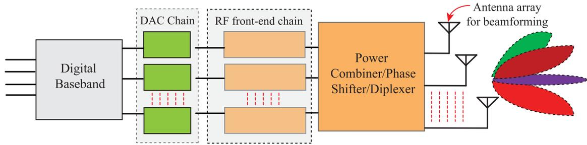
**FIGURE 9.** A simple example diagram of beam-forming based Massive MIMO 5G transmitter architecture: note the use of multiple antennas/antenna arrays. The PA will be a part of the RF front-end section. The massive MIMO based 5G receiver will also use antenna arrays.
