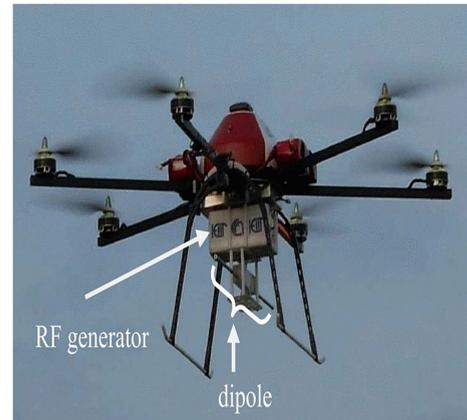
**FIGURE 16.** UAV based antenna radiation pattern measurement setup [216].
