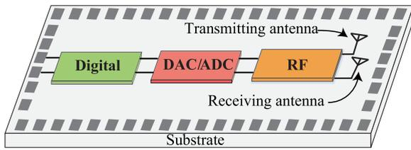
**FIGURE 1.** SoC based integration method: All sections of the wireless system including antennas are integrated on the same substrate, thus eliminating the need of lossy bond wires in contrary to other integration methods and resulting in a more compact, low loss, low power and cost-effective wireless modules.
