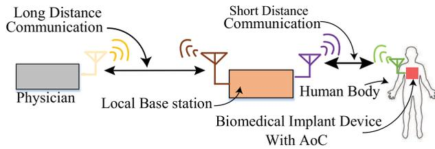
**FIGURE 17. Illustration of implantable biomedical device for patient's remote health monitoring with the help of AoC. Although one implant device has been shown here for the sake of simplicity, a large number of such devices will be inserted in the body to collect a variety of pathological and physiological parameters.**
