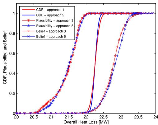
FIGURE 10. Comparison of plausibility, belief, pure probabilistic measures of the overall heat losses obtained by different approaches.
