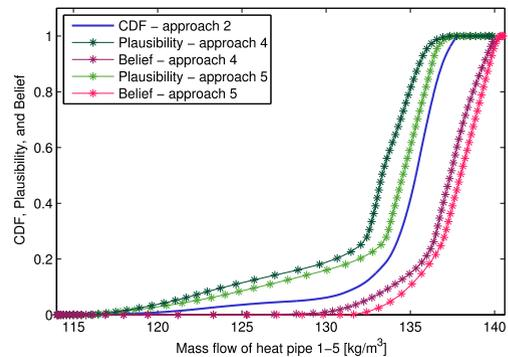
FIGURE 4. The cumulative probability distribution, plausibility, and belief of mass flow of heat pipe in the case 1.
