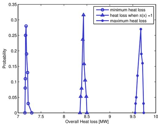
FIGURE 7. The PDF of membership function parameters of the overall heat loss in the case 1.
