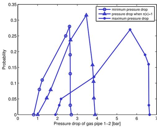
FIGURE 6. The PDF of membership function parameters of the pressure drop of gas pipe 1-2 in the case 1.
