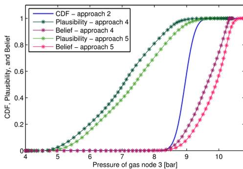
FIGURE 3. The cumulative probability distribution, plausibility, and belief of pressure of gas node 3 in the case 1.
