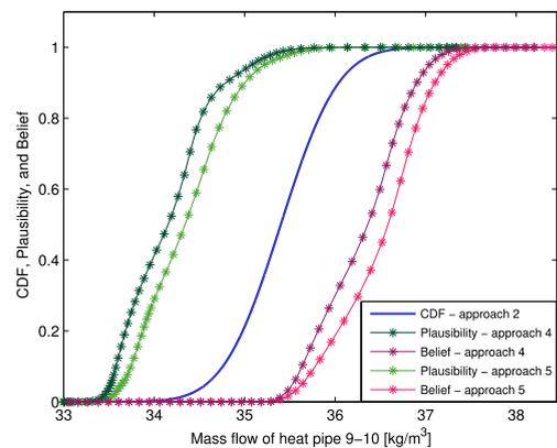
FIGURE 12. The cumulative probability distribution, plausibility, and belief of mass flow of heat pipe 9-10 in the case 2.
