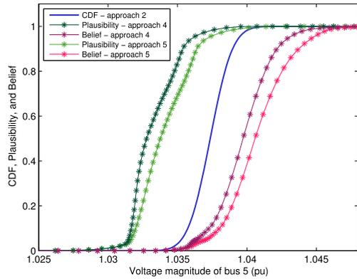
FIGURE 5. The cumulative probability distribution, plausibility, and belief of pressure of electrical bus 5 in the case 1.
