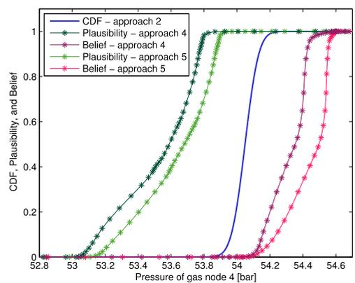
FIGURE 11. The cumulative probability distribution, plausibility, and belief of pressure of gas node 4 in the case 2.
