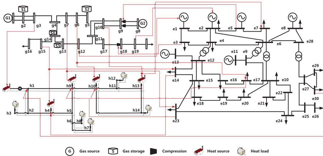
FIGURE 9. Schematic of the N20-H14-E30 MEC system.
