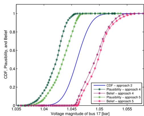
FIGURE 13. The cumulative probability distribution, plausibility, and belief of voltage magnitude of bus 17 in the case 2.
