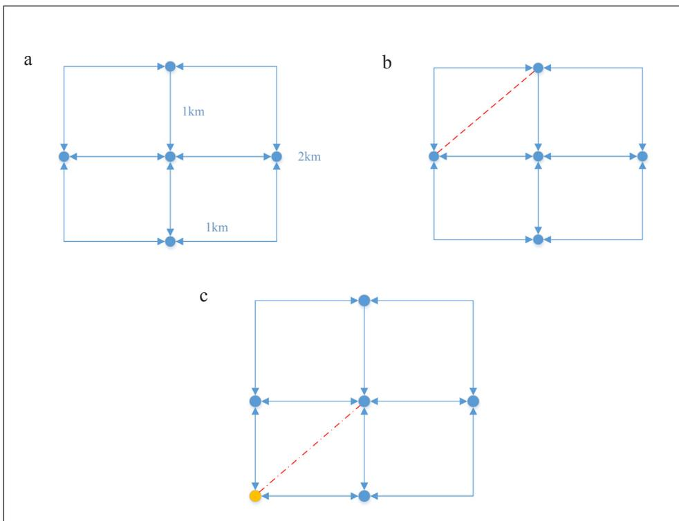
Fig. 1. A simple example to analyze travel cost variations. (a) Initial road network; (b) The first way to add a road; (c) The second way to add a road.
