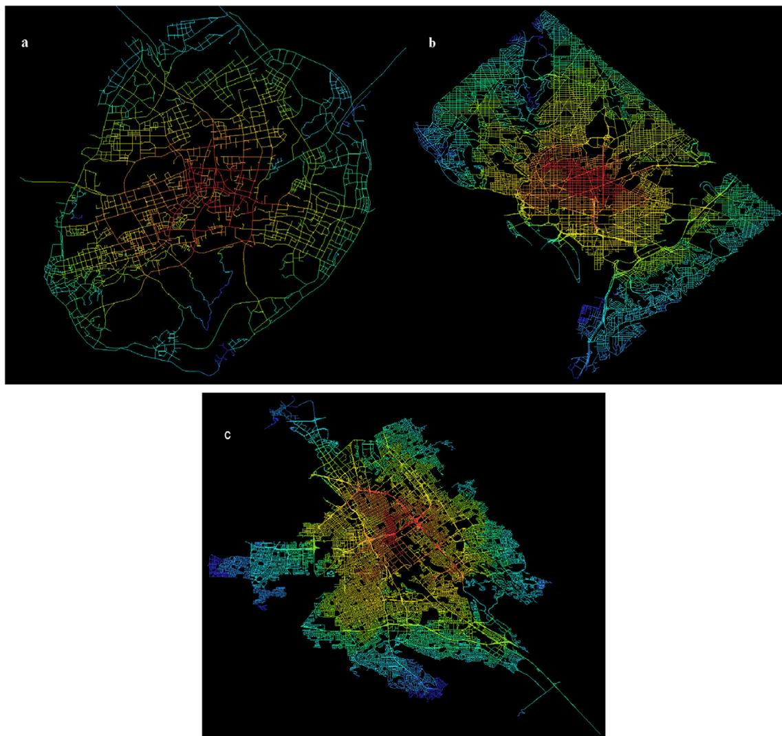
Fig. 4. Integration visualization of different road networks, (a) Xiamen, (b) Washington D.C., (c) San Jose. Values increase from blue to red.
