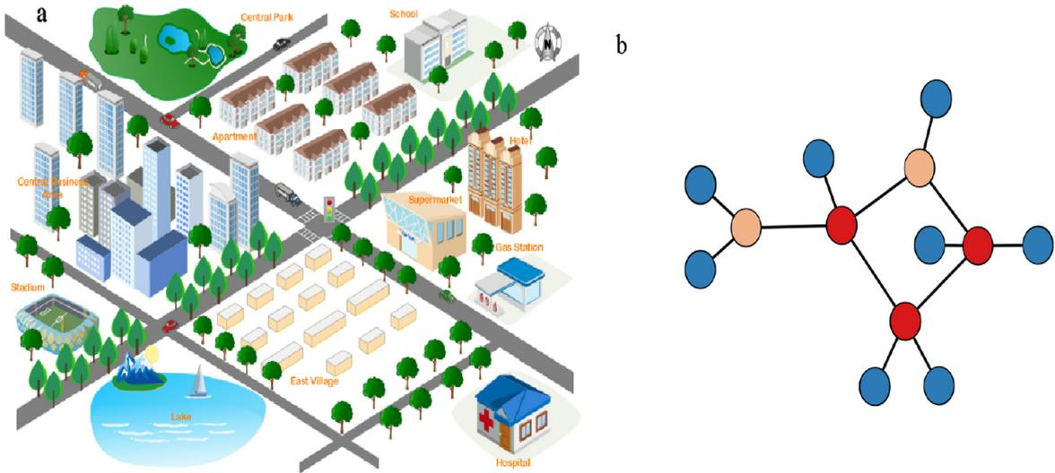
Fig. 3. Schematic diagrams of an urban road network: (a) real road network; (b) primal approach modeled network.
