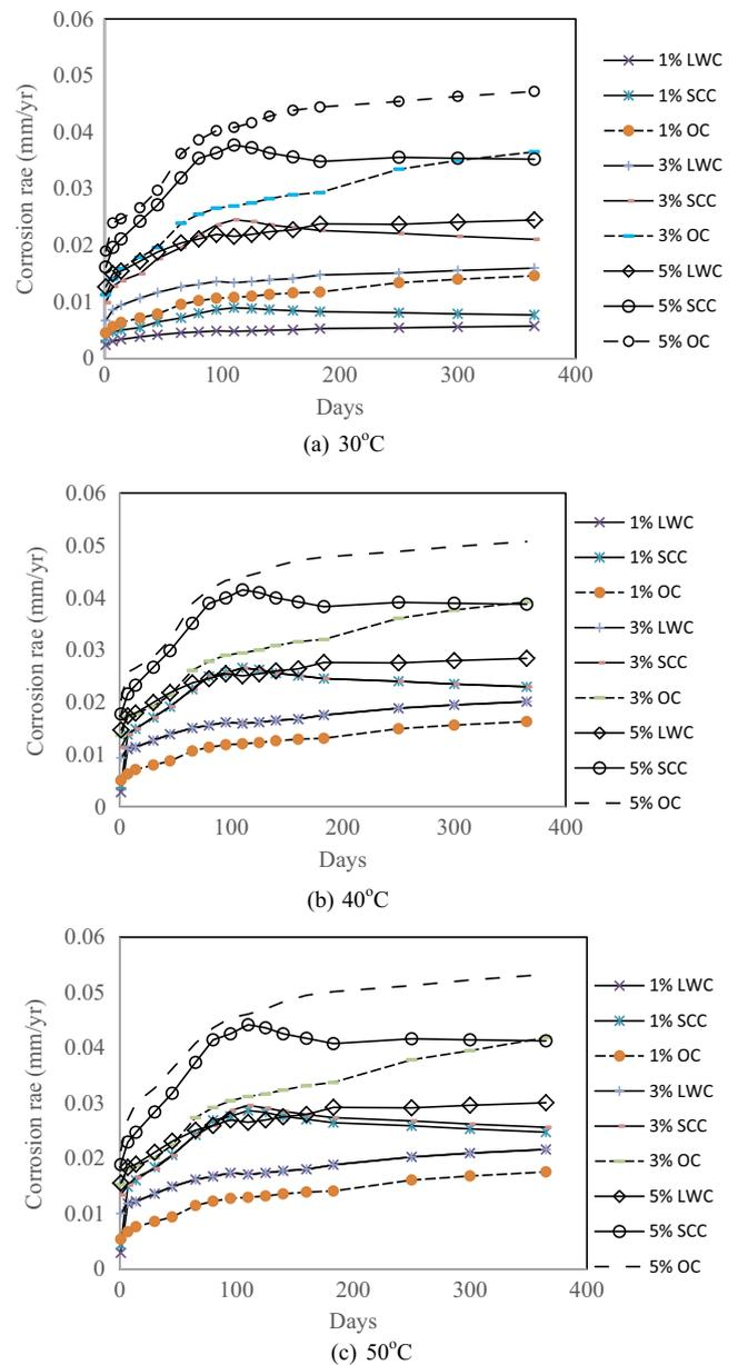
Fig. 2. Corrosion rates ( $I_{corr}$ ) of OC, SCC, and LWC specimens contaminated with 3% Cl kept.
