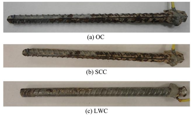
Fig. 4. Visual observation of corrosion of steel taken out from various specimens.
