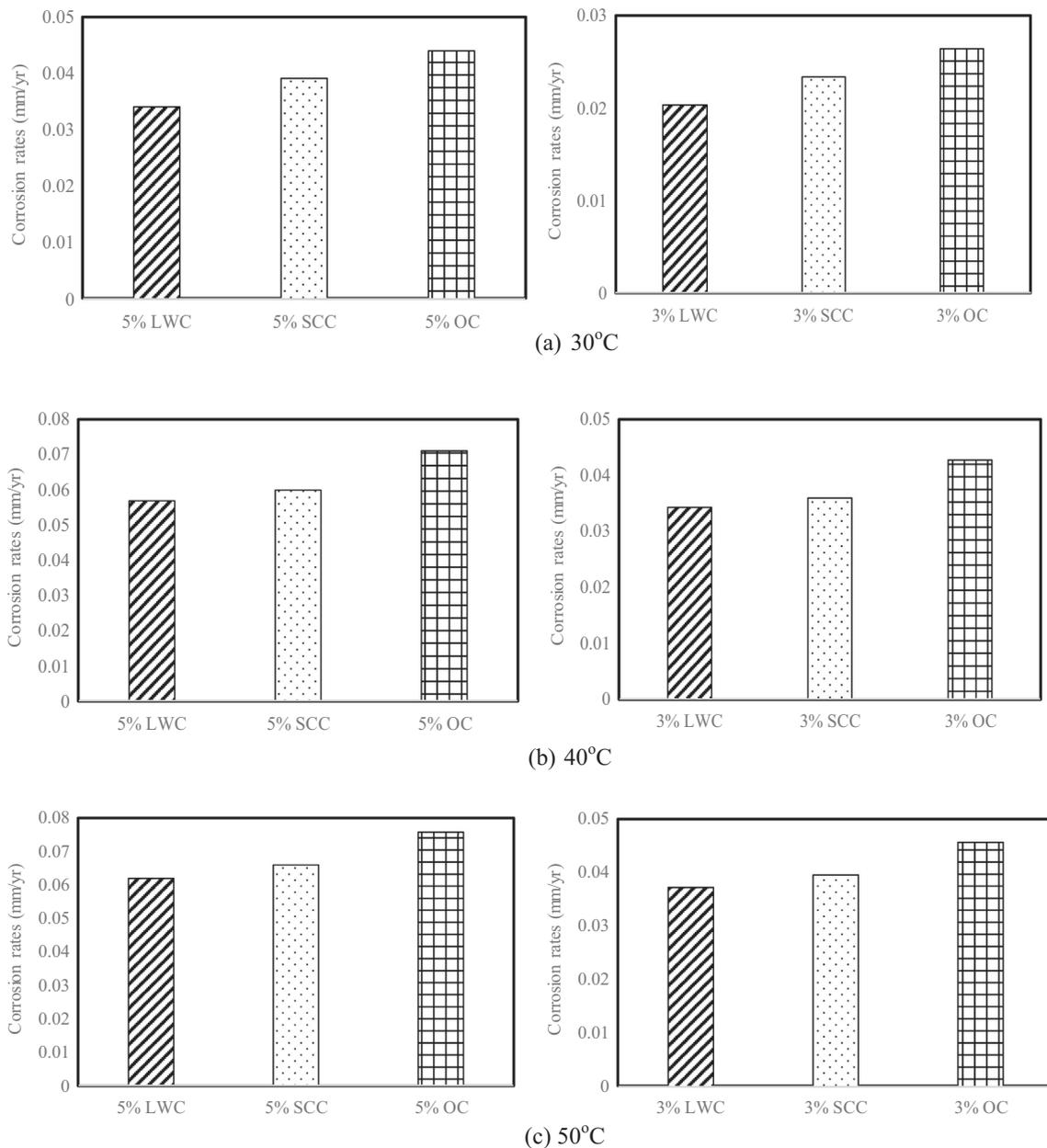
**Fig. 5.** Corrosion rates (mass loss) of specimens after 365 days in varying chloride ((a)–(c) 3 and 5%, (d)–(f) 1%), and temperature exposures ((a) 30 °C, (b) 40 °C, (c) 50 °C, (d) 30 °C, (e) 40 °C, (f) 50 °C).
