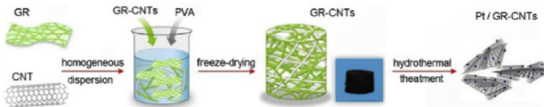
Fig. 18. Production process of GR-CNTs and Pt / GR-CNTs.
