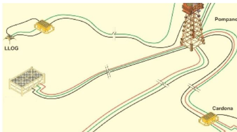
Fig. 23.7 Pompano subsea tieback schematic.
