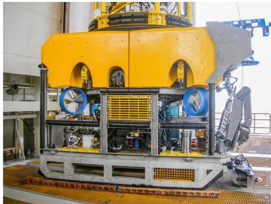
Fig. 23.12 Work class ROV sitting on vessel's deck.
