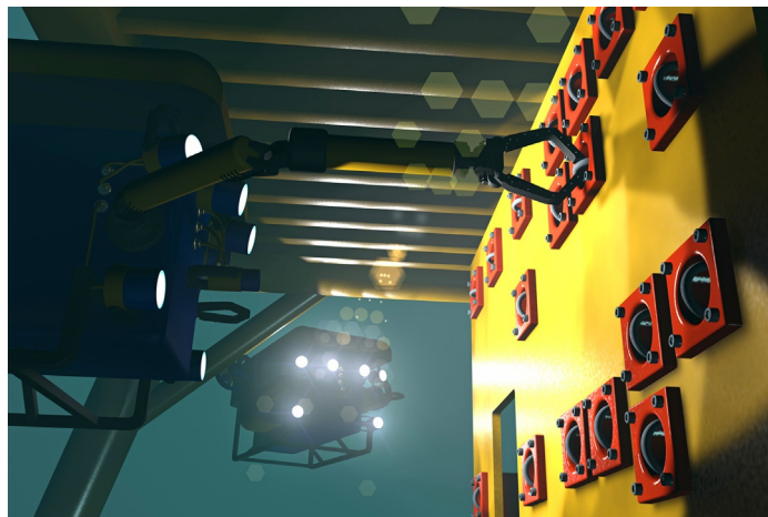
Fig. 23.14 Rendition of ROV manipulating subsea wellhead controls under a steel structure.
