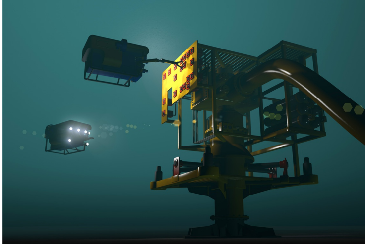
Fig. 23.13 Rendition of ROV manipulating a control valve on a subsea wellhead.
