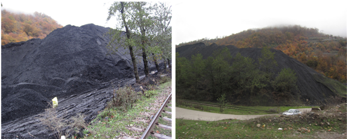
Fig. 2. Deposit of untreated coal waste in Alborz Markazi coal washing plant.
