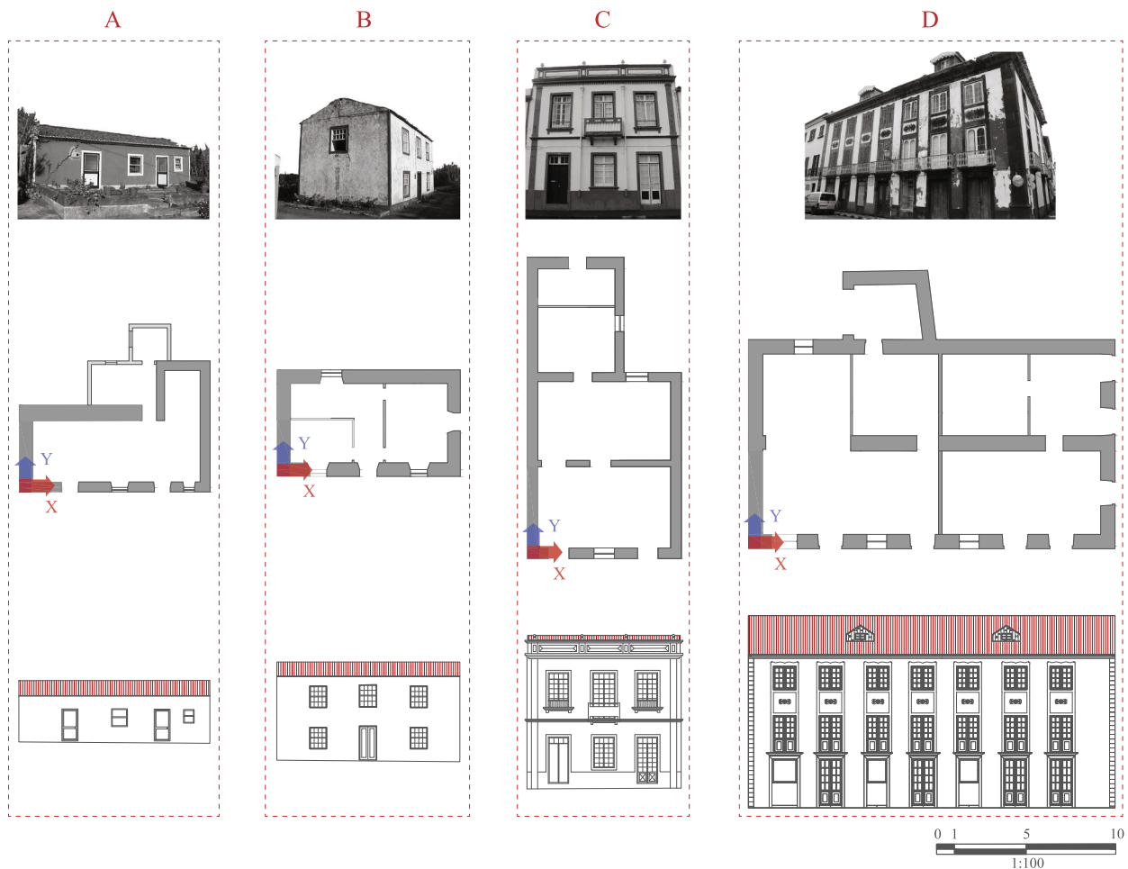
Fig. 2. Overview of the geometry and building typology of each case study (from A to D): ground floor plans and the respective main façade elevations. Please note that traditional stone masonry elements are coloured in grey, while masonry brick blocks are coloured in light grey. Moreover, the reference axes (X and Y) considered throughout the paper to each model are identified in the respective ground floor plans.
