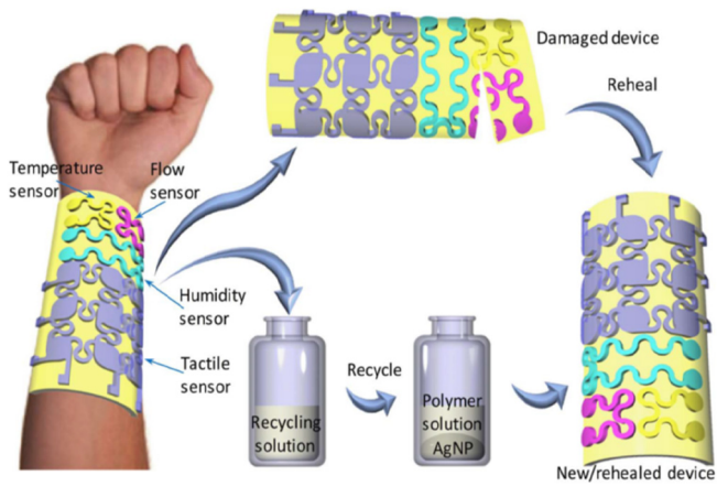
Fig. 9. Schematic of the rehealability and recyclability of an E-skin. When moderately damaged, the E-skin can be rehealed. The rehealed E-skin can restore mechanical and electrical properties to levels comparable with those of the original device. When severe damage occurs or the device is no longer needed, the whole E-skin can be completely recycled, leaving no waste. Once recycled, a short-oligomer/precursor solution and Ag nanoparticles that can be used to make new materials and devices are obtained. 105
