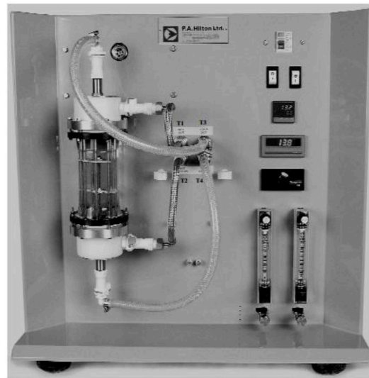
Fig. 1. The H101C heat exchanger [16].
