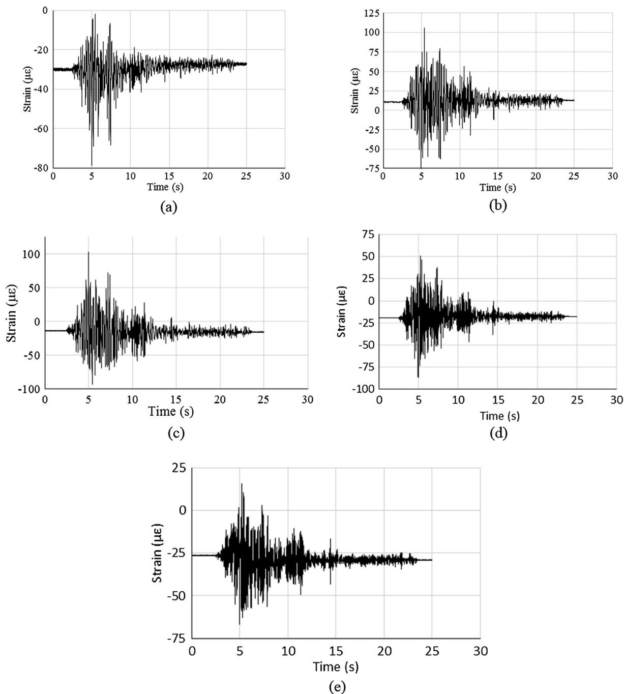
**Fig. 16.** Strain time-history curve of lining at left sidewall foot for different monitoring sections. (a) Strain time-history curve of lining at section 1-1; (b) Strain time-history curve of lining at section 2-2; (c) Strain time-history curve of lining at section 3-3; (d) Strain time-history curve of lining at section 4-4; (e) Strain time-history curve of lining at section 5-5.
