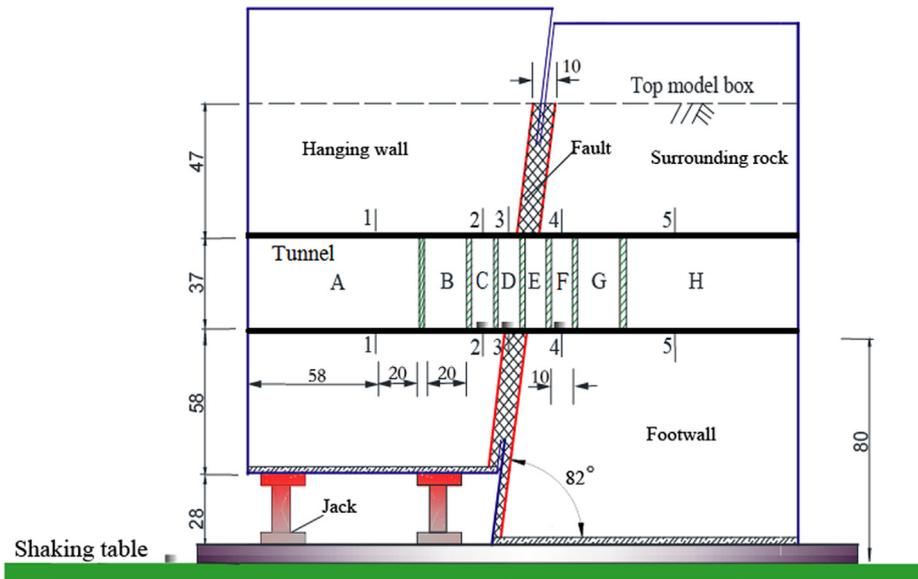
Fig. 8. Distribution of monitoring section and sectional tunnel lining for model box (unit: cm).
