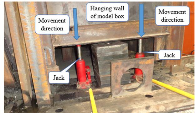
**Fig. 11.** Four jacks of hang wall bottom for model box.
