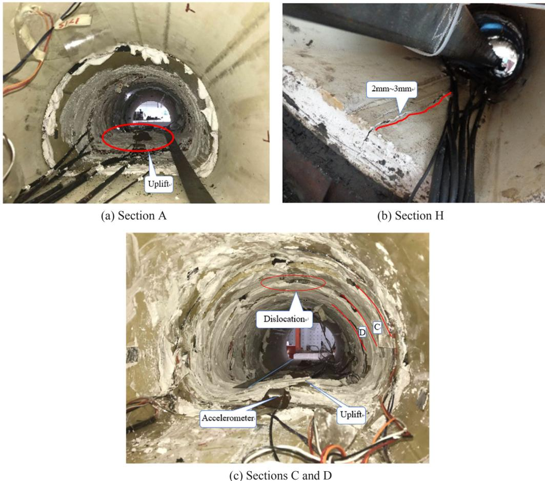
Fig. 14. Cracking distribution of tunnel lining after normal fault movement.
