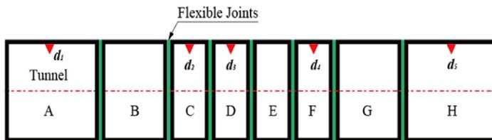
(a) Displacement sensors distribution of sectional tunnel lining
