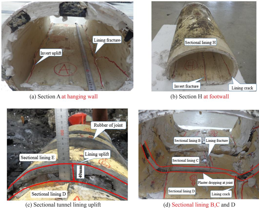
Fig. 15. Failure mode of tunnel lining after shaking table test.
