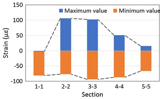
Fig. 17. Strain maxima and minima of sidewall foot for different monitoring sections.
