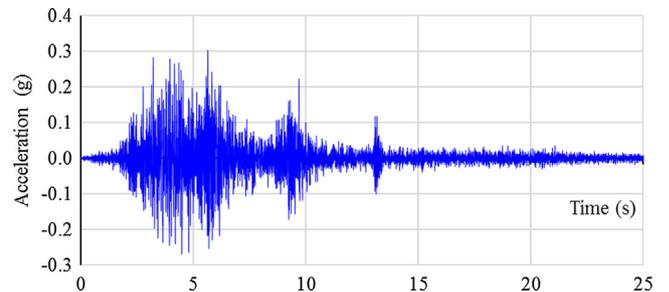
**Fig. 12.** Input earthquake wave recorded from the bedrock.
