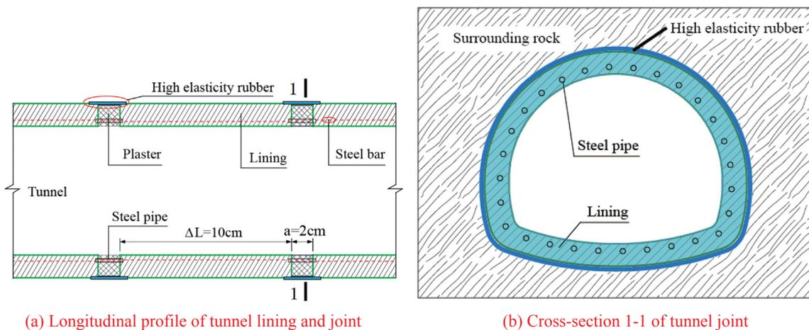
(a) Longitudinal profile of tunnel lining and joint
