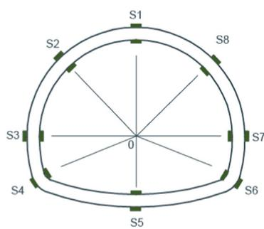
(c) Strain gauges distribution of sections 2-2, 3-3 and 4-4
