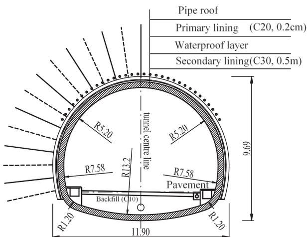
Fig.7. Cross-section of tunnel structure for test (unit: m).
