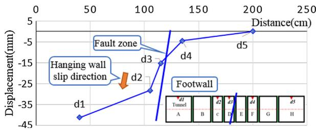
Fig. 13. Longitudinal deformation curve for sectional tunnel linings after fault movement.
