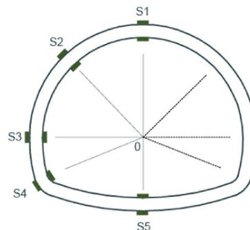
(d) Strain gauges distribution of monitoring sections 1-1 and 5-5
