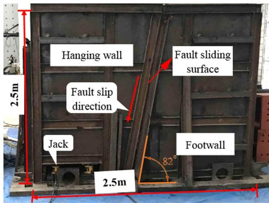
Fig. 6. Shaking table model box with fault.
