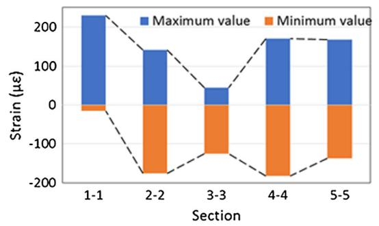
Fig. 19. Maximum and minimum strain values of arch shoulders for different monitoring sections.
