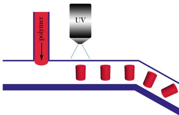
*Figure 2 Schematic illustration of the preparation of nonspherical particles using a microfluidic system. The outlet channel defines particle shape.*
