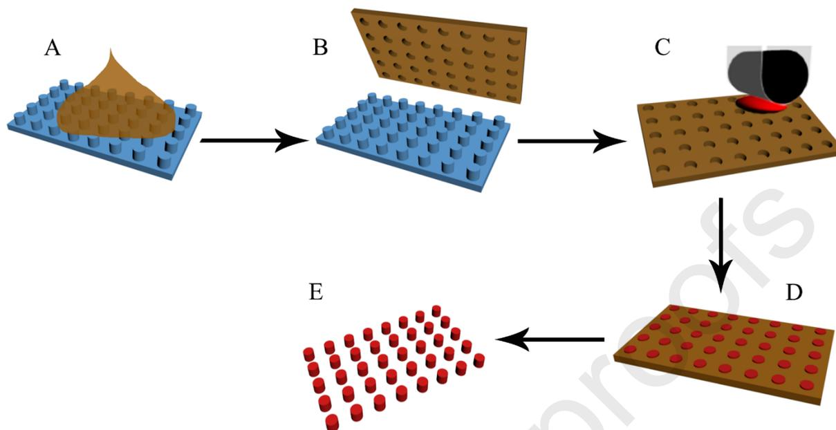
*Figure 3 Schematic illustration of PRINT method process: (A) a liquid polymer mold (brown) is delivered onto a silicon master with desired shape and size (blue); (B) polymer is peeled away to generate a mold with cavities; (C) roller is brought into contact with particle solution and the mold; (D) particles are cured in the mold; (E) nonspherical particles with desired shape and size are harvested.*
