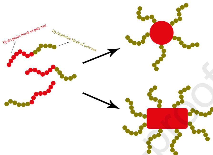
*Figure 1 Schematic illustration of self-assembling method: Hydrophilic and hydrophobic blocks of polymer are self-assembled to form nonspherical particles.*
