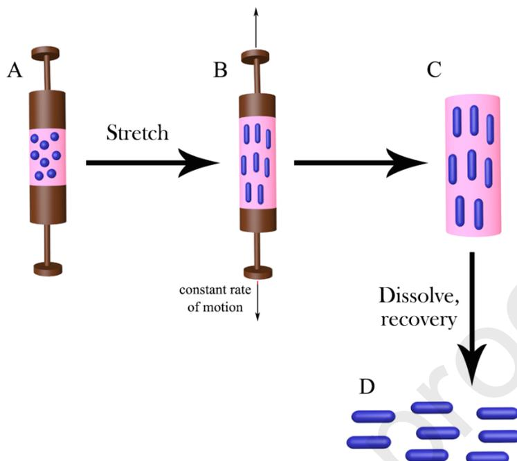
*Figure 4 Schematic illustration of film stretching method process: (A) liquefaction of spherical particles by using heat or a solvent; (B) stretching the film in one or two dimensions; (C) eliminating the motion; (D) dissolving the film forming material and harvesting the nonspherical particles.*
