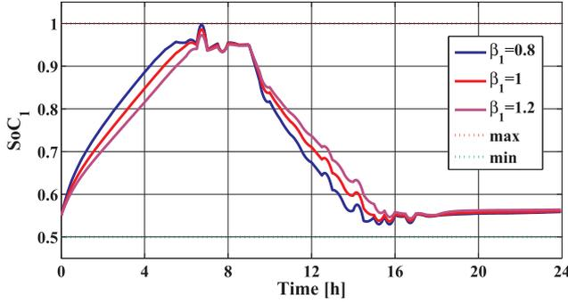
Fig. 14. Scenario 3:  $SoC_1$  of the battery, as defined in (35a), with proportional uncertainties of the battery voltage parameter as in (39).
