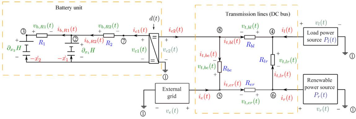
Fig. 2. Electrical circuit of the DC microgrid.
