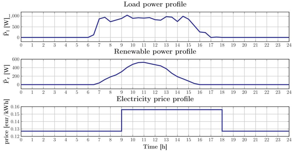
Fig. 4. Profiles of load, renewable power and electricity price.
