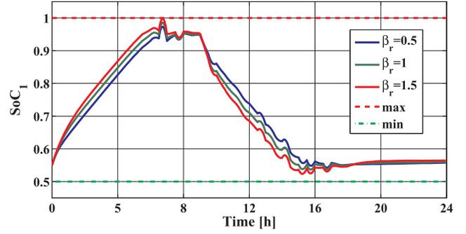
Fig. 16. Scenario 5:  $SoC_1$  of the battery, as defined in (35a), with proportional uncertainties of the resistors as in (41).
