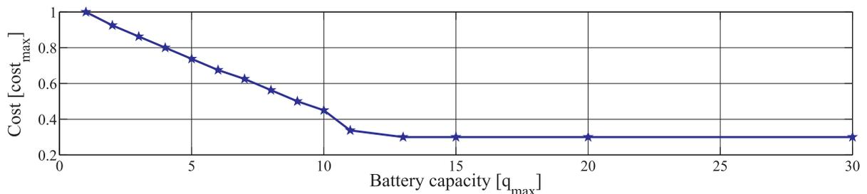
Fig. 8. Nominal scenario: cost and battery capacity relation.
