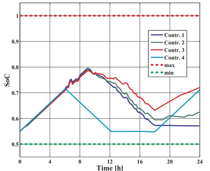
**Fig. 21.** Battery charges corresponding to different controllers with  $i_{b,max} = 5A$ .
