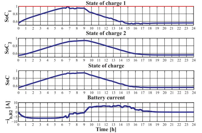
Fig. 9. Nominal scenario: battery state of charges ( $SoC_1$ ,  $SoC_2$ ,  $SoC$  as defined in (35)) and discharge current.
