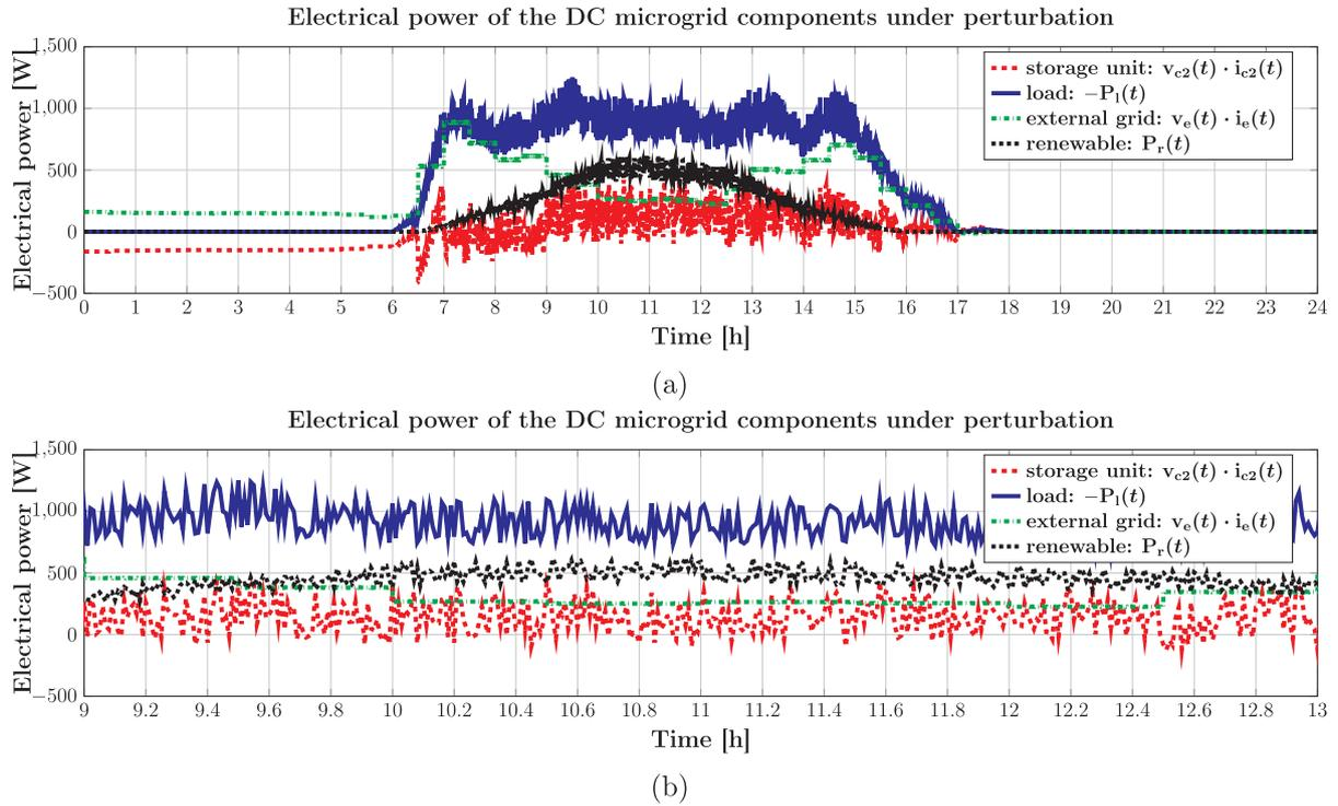
Fig. 11. (a) Scenario 1: actual electrical power charged/discharged by the DC components under perturbation scenario. (b) Zoom for the subfigure (a).
