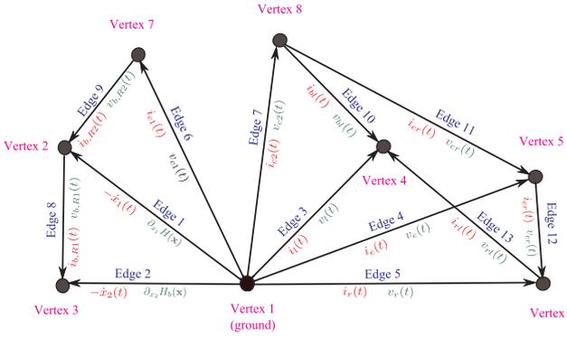
Fig. 3. Directed graph corresponding to the DC microgrid circuit.
