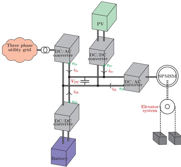
Fig. 1. DC microgrid elevator system.
