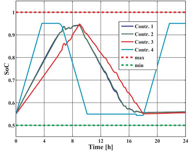
**Fig. 20.** Battery charges corresponding to different controllers with  $i_{b,max} = 20A$ .
