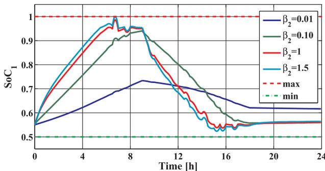
Fig. 15. Scenario 4:  $SoC_1$  of the battery, as defined in (35a), with proportional uncertainties of the battery capacity parameter as in (40).
