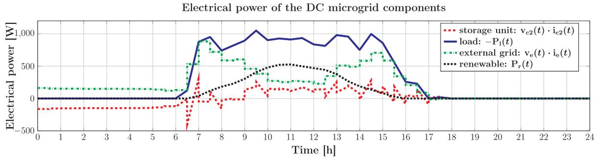
Fig. 7. Nominal scenario: actual electrical power charge/discharge by the DC components.
