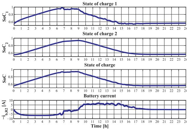
Fig. 12. Scenario 1: battery state of charges ( $SoC_1$ ,  $SoC_2$ ,  $SoC$  as defined in (35)) and discharge current (perturbation scenario).
