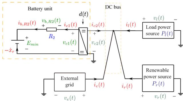
Fig. 19. Electrical circuit of the DC microgrid reduced model.
