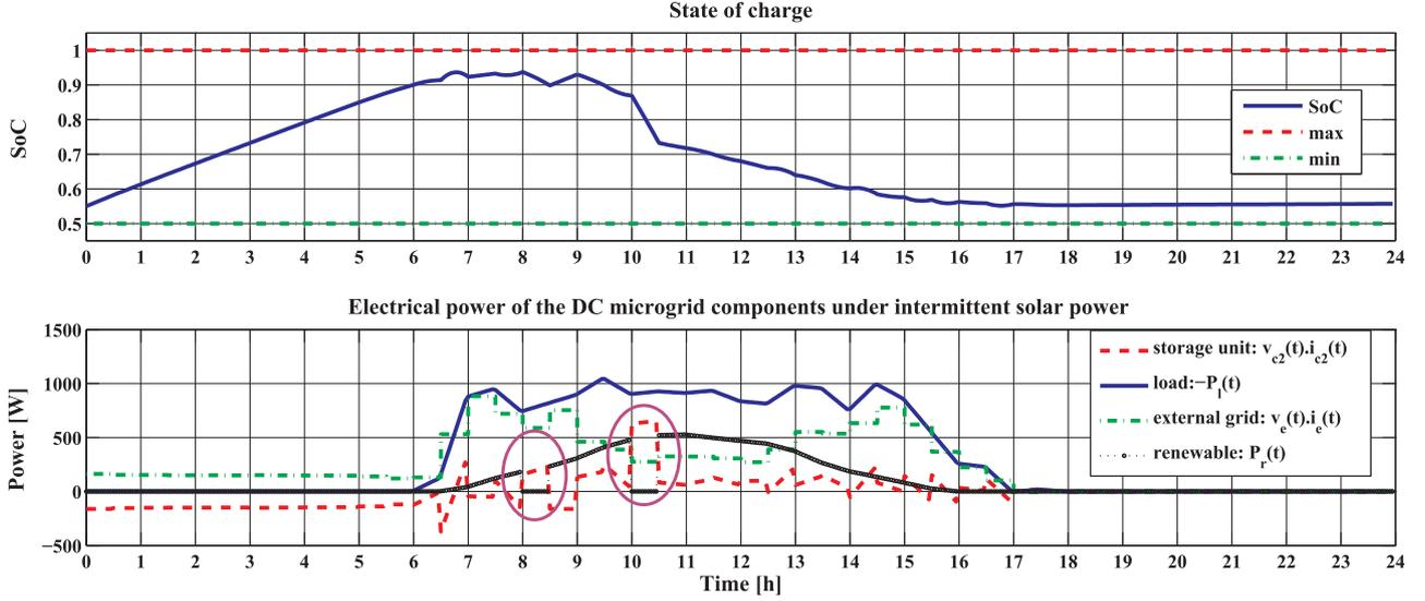
Fig. 17. Scenario 6: battery SoC in (35b) and electrical power of the DC microgrid components under the intermittent renewable power.
