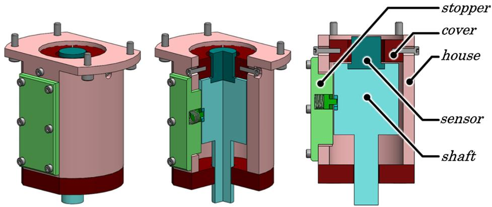
Fig. 3. One structural design alternative,  $d_{SEP}$  with two adjustment mechanisms, for the sample product.
