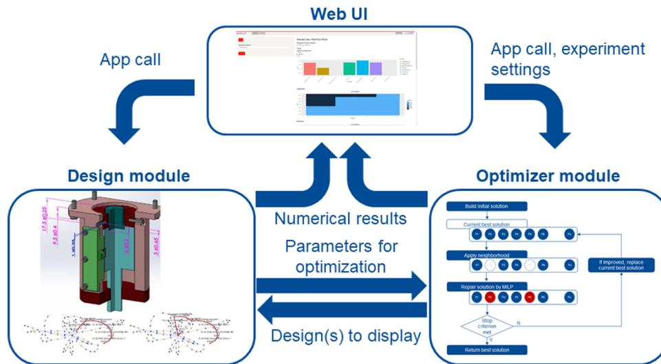
Fig. 7. System architecture of the proposed decision support system.
